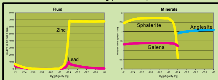
FIG.5 This different behaviour displayed by Zn and Pb at low oxygen fugacity is a consequence of the precipitation of anglesite, without formation of any Zn-bearing mineral. This caused the fluid to be enriched in Zn relative to Pb.
