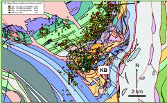
•A map of the mica crystallinty index shows that highly crystalline micas occur in the core of the phengite cell. Low crystallinity white micas occur around the edges.
