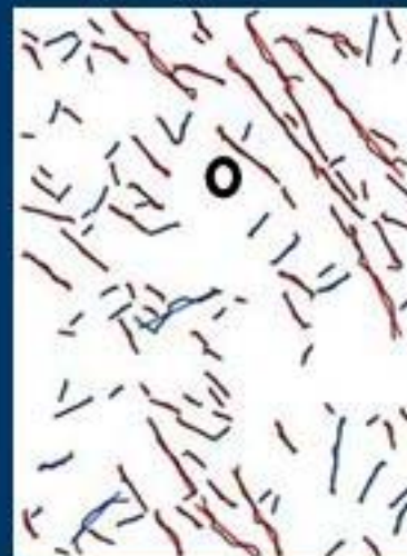
Structure - conjugate NW & NE worm/fault network
