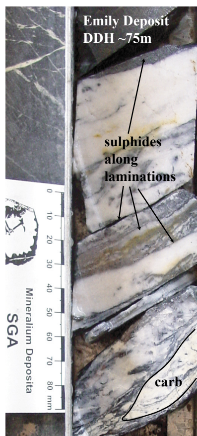
Fig. 3.7: Mineralised laminated quartz veins in drillcore from the Emily deposit.
