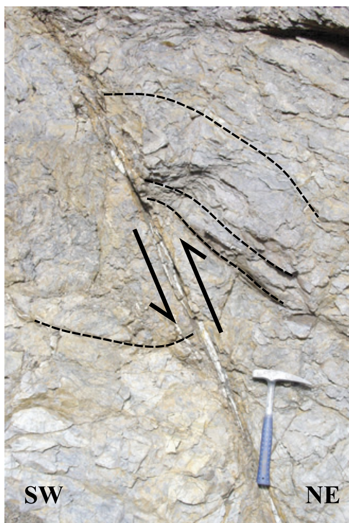
Fig. 2.5: Outcrop photograph of NW-striking, quartz-filled _{ab}D_3 reverse fault in pit wall at the Camel Creek deposit. Dashed lines represent fault drag. Hammer for scale.
