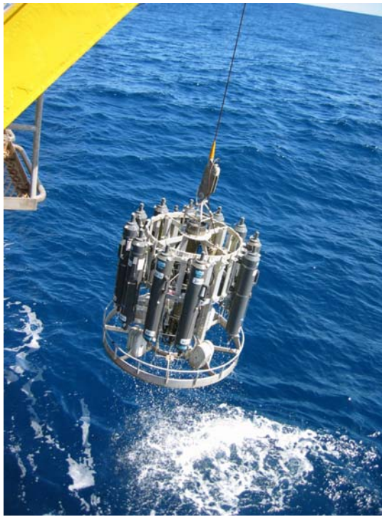
Figure 4.11. Photograph of CTD rosette deployed from starboard A-frame. Niskin bottles were attached to the rosette to collect water samples from the water column.
