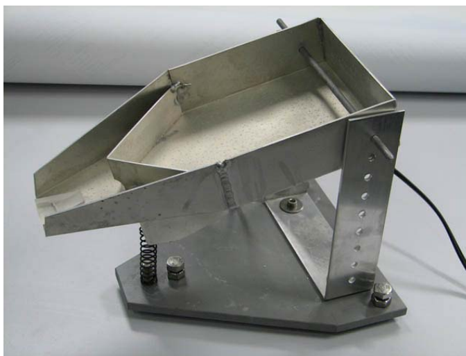
Figure 8.1. Crook wet sediment splitter used to evenly divide (split) boxcore elutriate during post-processing of infauna.
