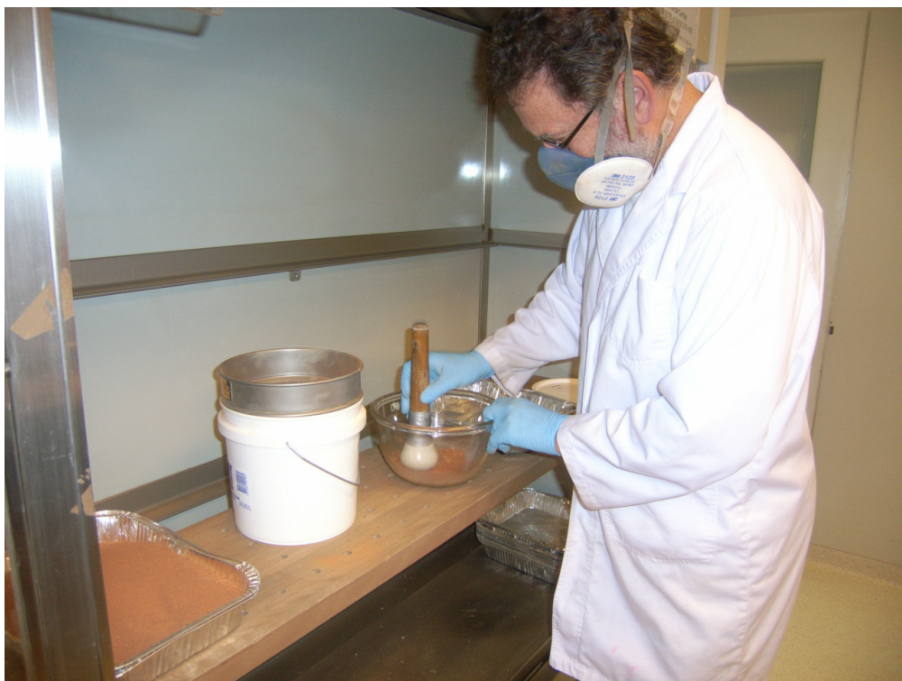
Figure 13. Disaggregating clay clumps in a sample with a porcelain pestle to ensure it passes through the 3.35 mm stainless steel mesh.
