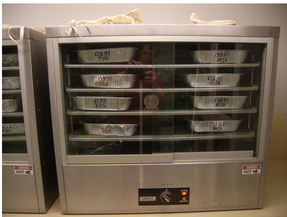
Figure 12. Drying of the samples in thermostatically controlled fan-forced ovens at 40 ( \pm 5 ) °C. Note the calico bags on top of the oven; they follow each sample through the process to minimise mislabelling risk.
