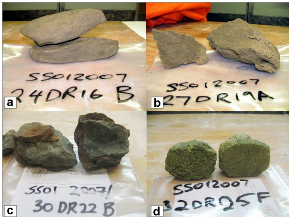
Figure 4.16. Examples of sandstone recovered during the Bight survey: a) fine, micaceous sandstone, b) fine sandstone, c) fossiliferous, ferruginous fine sandstone and d) glauconitic sandstone (greensand).
