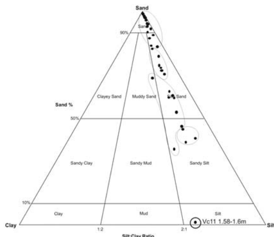
Figure 18 : The graphs show the grainsize distribution of sub-samples from the vibracores. Four different grainsize distributions are shown on the graphs; silt, very fine sand, fine to medium sand and sandy clays. Within the grainsize distributions they can be further separated into facies by \text{CaCO}_3\% - samples with high \text{CaCO}_3\% are highlighted by a thicker line. VC11-1.58-1.6m is highlighted on the graph of sandy clays by a dashed thick line.
