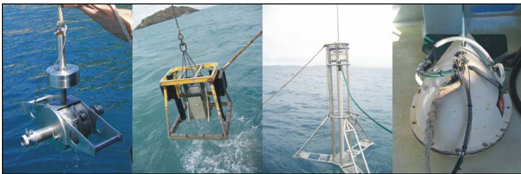
Figure 3: Shipeck sediment grab sampler, box-corer, vibracorer (3 m configuration), the James Cook University Datasonics “Chirp” sub-bottom profiler towfish (Datasonics, 1999).
