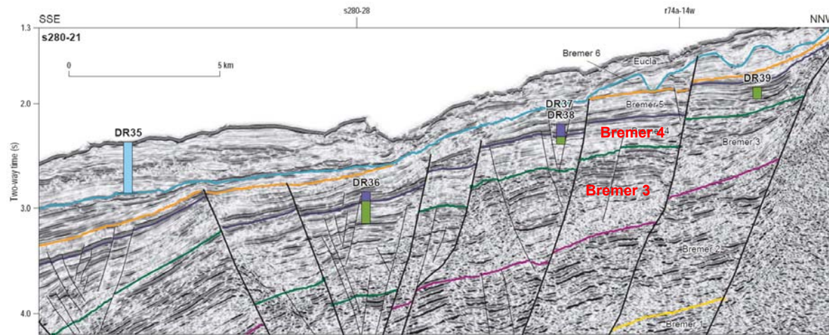
Geoscience Australia seismic line S280-21 showing the nature of Bremer-4 (Extension-2) package in the Bremer Sub-basin (from O'Leary et al., 2005).
