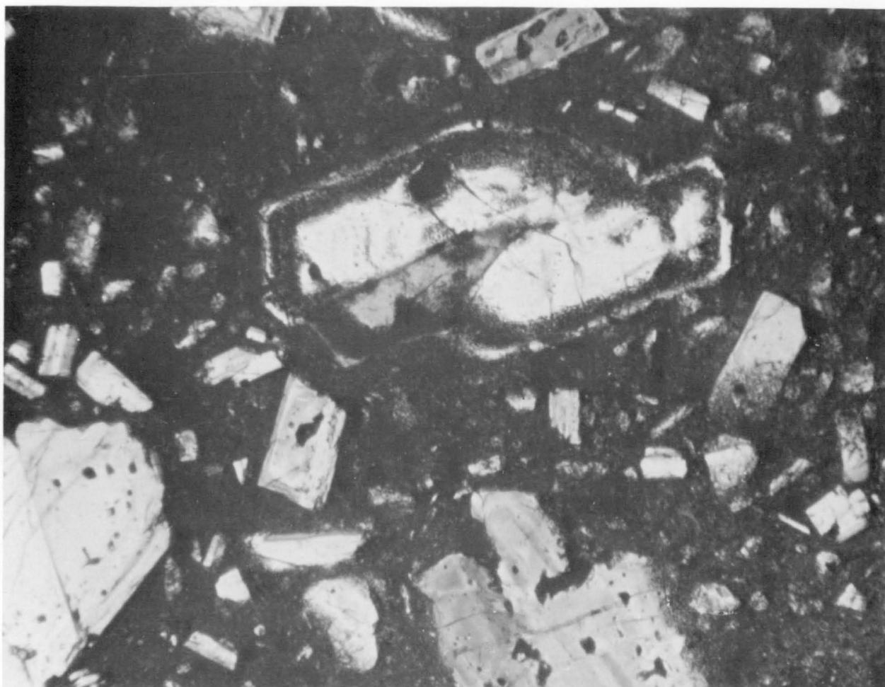
Fig. 8. Photomicrograph of Jaulu Volcanics andesite showing corroded zone of plagioclase phenocryst and aphanitic groundmass (M/1117).
