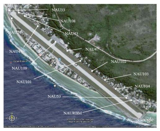
After reduction an internal precision of 1mm  $\sqrt{K}$  or better was achieved, where K is levelled distance in kilometres. Project Specification for precision is 2mm  $\sqrt{K}$ .
