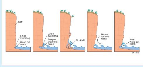
Stages in erosion of a cliff by waves.
