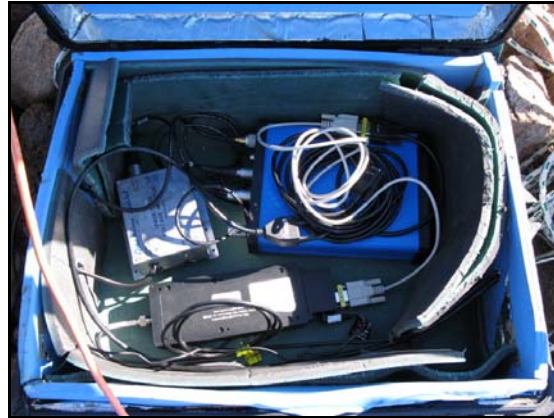
Figure 37: Grove Mountains, inside GPS receiver / modem case.
