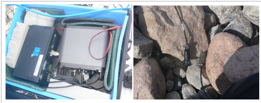
Figure 10 and 11: Left: Wilson Bluff, pelican case containing receiver and computer. Right: receiver power cable on arrival.
