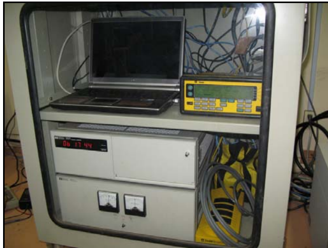
Figure 78: Primary GPS computer and Trimble receiver equipment indoors
