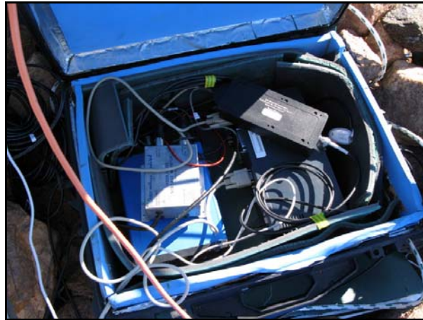
Figure 28: Grove Mountains, inside receiver / computer pelican case.
