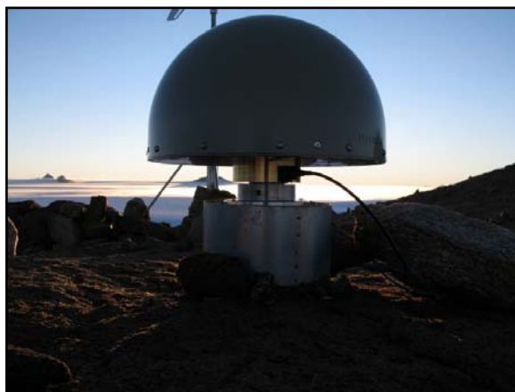
Figure 29: Grove Mountains, survey monument (AUS351) and GPS antenna
