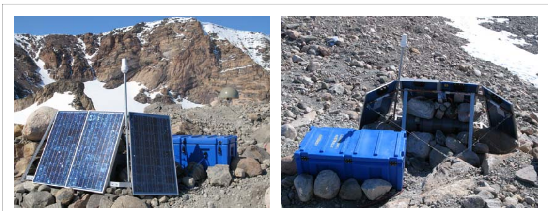
Figure 16 and 17: Wilson Bluff, repositioned and repaired solar panel frame, modem antenna, primary battery box and GPS antenna, view south (left) and view north (right).
