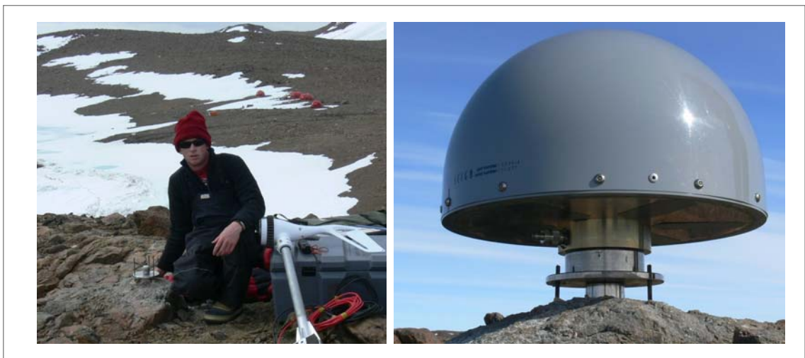
Figure 1 and 2: Left: Bunger Hills, Nick next to survey mark (Photo looking North with apple huts in background). Right: Bunger Hills, antenna with snow dome attached.
