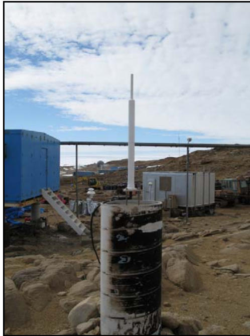
Figure 76: DORIS beacon, view south east, towards VLBI dome
