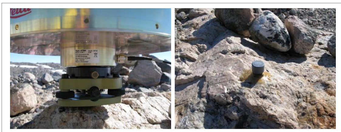
Figure 23 and 24: Left: Antenna and tribrach over WBF0. Right: WBF0 close up view.
