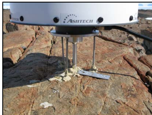
Figure 42: Dalton Corner, close up of survey monument.
