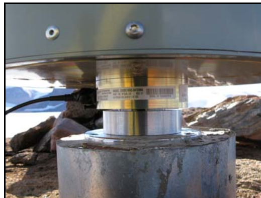
Figure 36: Grove Mountains, survey monument (AUS351) and GPS antenna.
