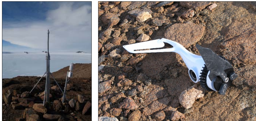
Figure 16: Wind turbine stand (left) and damaged wind turbine (right).
