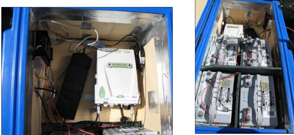
Figure 33: Receiver and Iridium Data Modem (left) and equipment box after equipment upgrade (right).
