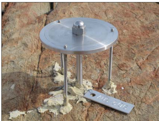
Figure 46: AUS306 survey monument remaining at site (left); Small rock cairn indicates the location of the Dalton Corner site (right).
