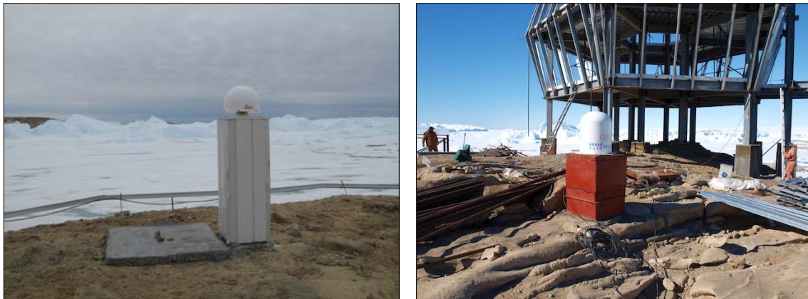
Figure 36: New CHINARE CORS ZHON at Zhong Shan (left) and old Zhong Shan CORS, it was moved due to the obstruction of the new atmospheric physics building (right).
