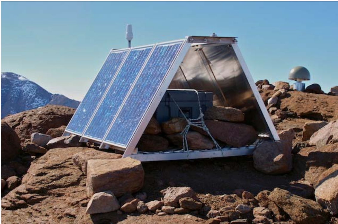
Figure 11: Solar panel frame structure, as installed at the Grove Mountains (December 2009).
