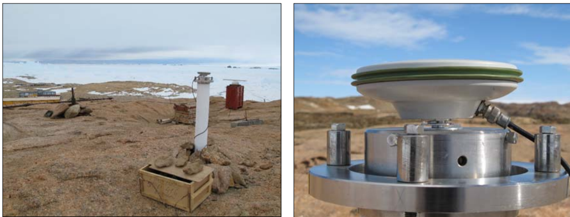
Figure 37: New Russian CORS at Progress II (left) and close up view (bottom right).
