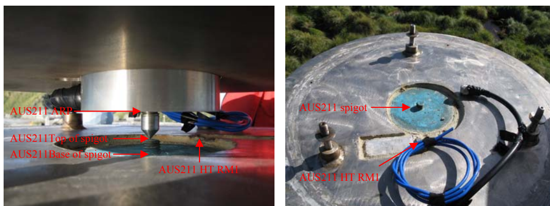
Figure 42: Macquarie Island ARGN pillar height reference points, plan and profile view.
