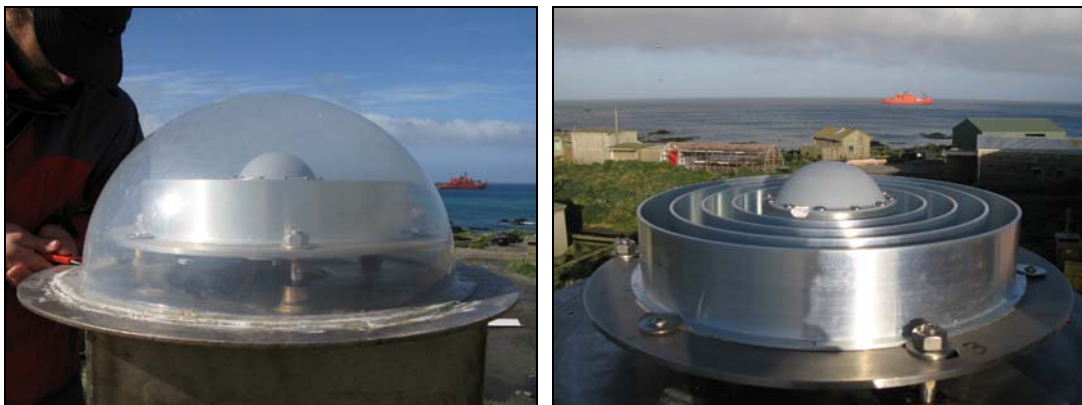
Figure 8: Macquarie Island ARGN GPS antenna, dome and bracing mount
