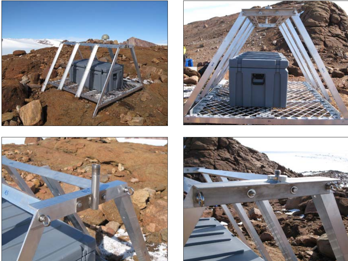
Figure 24: Top Left and right: Solar panel frame and equipment box; Bottom Left: Iridium antenna support and connection; Bottom Right: Wind turbine connection, with adjustable support.
