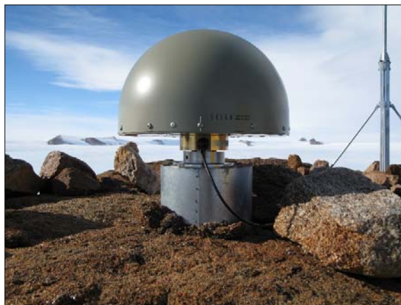
Figure 19: Survey Monument (AUS351) and GPS antenna
