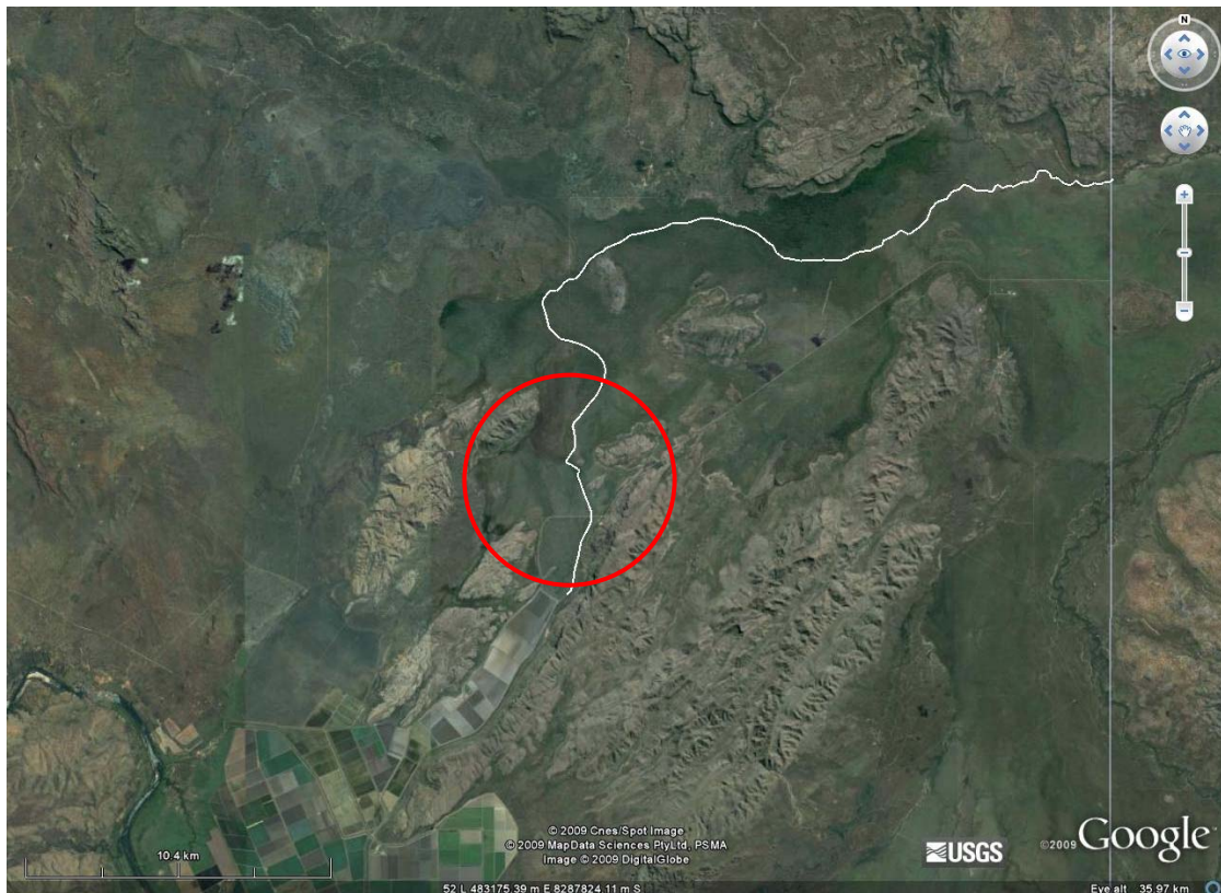
Figure 359: Google earth image showing the location of the D8 swamp, which is driven by discharge of over 3Gl/yr discharge from the D8 drain. The water body has become a semi-permanent wetland (dark brown area highlighted) formed by the terminus of the M1 supply channel. To the south of the wetland, the M1 channel is denoted by the white line. To the north, the white line denotes the natural drainage line. A blow-up of the wetland area is shown in Figure 142.
