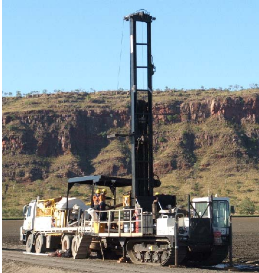
Figure 29: The sonic rig on site at hole O4.
