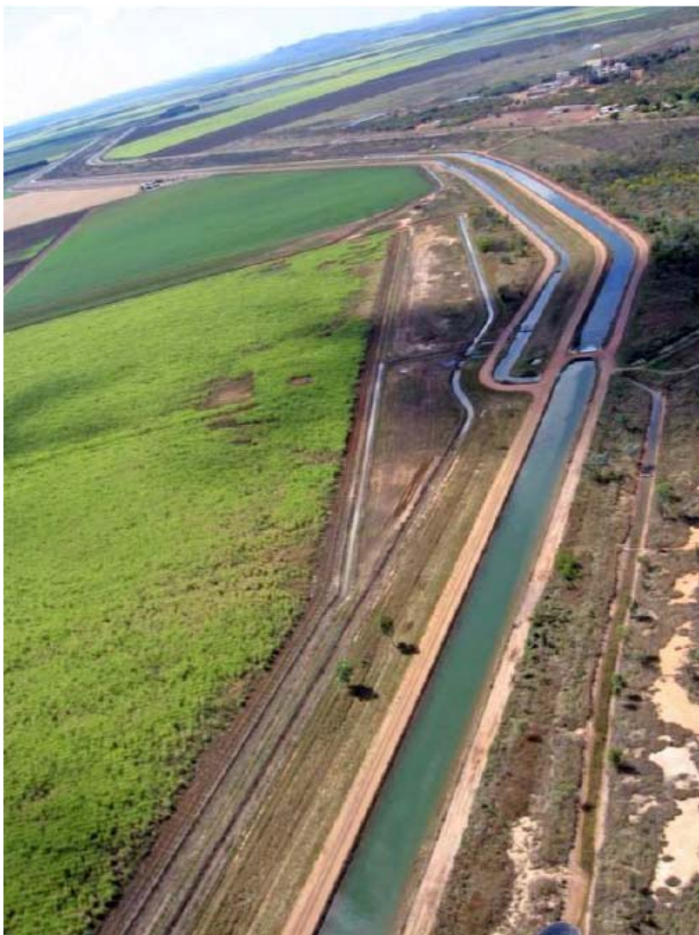
Figure 297: Aerial photograph showing location of seepage from the M1 supply channel, adjacent to areas of bare ground and reduced crop productivity (mangos) that corresponds with areas of locally high watertables (when the supply channel is filled) and high groundwater and sub-soil salinities. Photograph from Smith & Price (2008).
