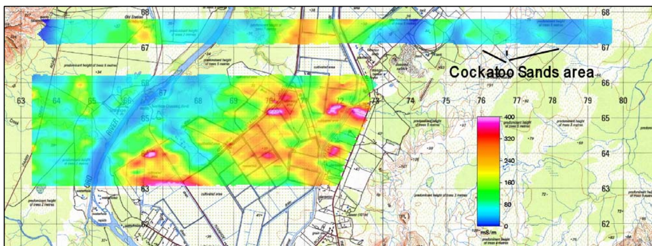
Figure 314: 0-2m interval conductivity from a fast approximate inversion of the SkyTEM data over part of ORIA and the Cockatoo Sands area.
