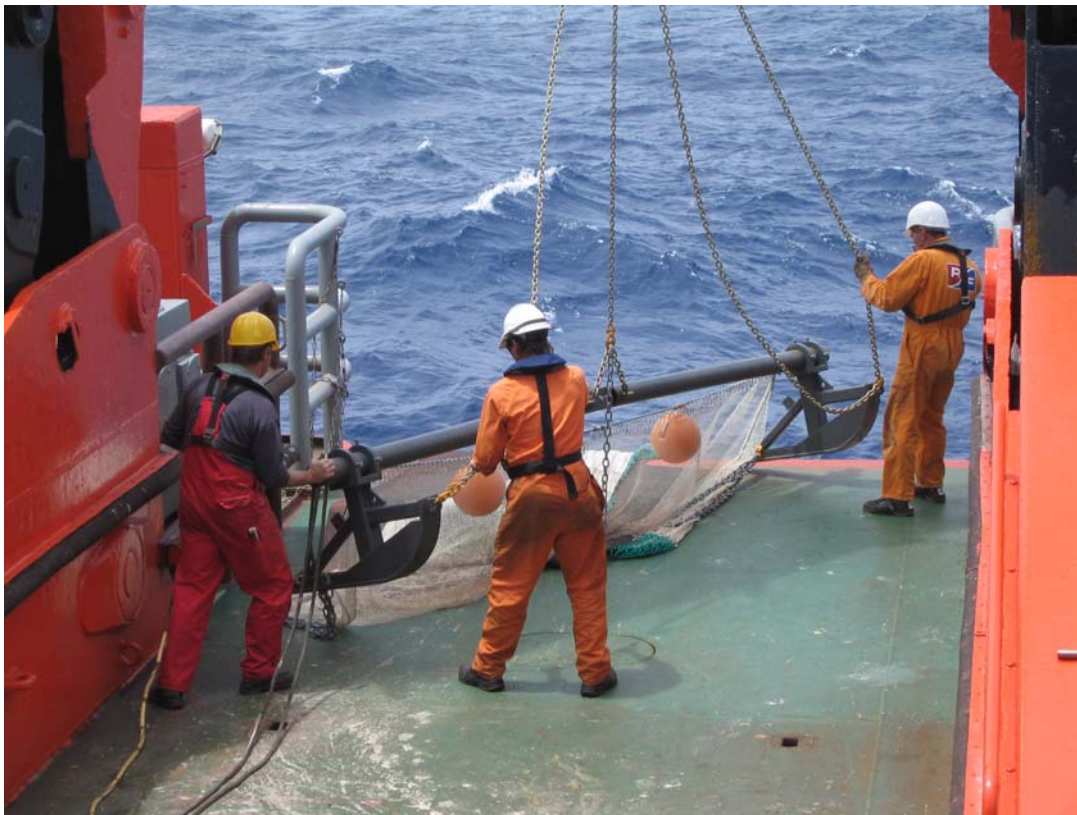
Figure 3.8. Photo of the deployment of the beam trawl off the aft deck.
