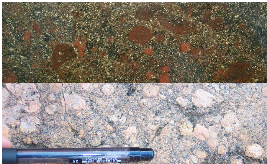
Figure 4-4: Top – typical Ernest Henry ore breccia with hematite-Kfeldspar altered clasts in a magnetite- chalcopyrite-pyrite-Kfeldspar-calcite±barite-titanite matrix. Bottom – typical breccia from a breccia pipe emanating from the Mt Angelay Granite and crosscutting Soldiers Cap Group schists, from the western edge of the Snake Ck anticline, with albite-actinolite-magnetite±Kfeldspar-chlorite clasts set in a albite-magnetite-hematite-actinolite matrix Scale is similar in both photographs..
