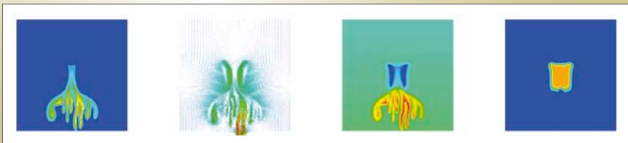
Figure 3: Patterns of salinity, fluid flow vectors, fluid density and temperature due to thermohaline convection. Model is initialised with an internal box of higher salinity, lower temperature fluid. See Section 2.4 for details.
