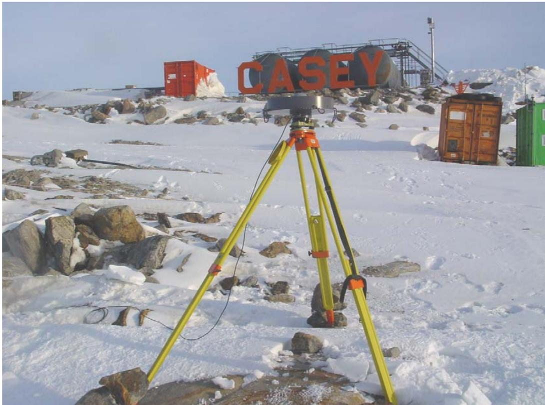
*Figure 4.1. GPS antenna over the TGBM (AUS299)*
