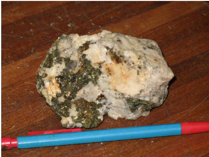
Fig. 20. Sample of northwest-trending dolomite-quartz-chalcopyrite vein .
