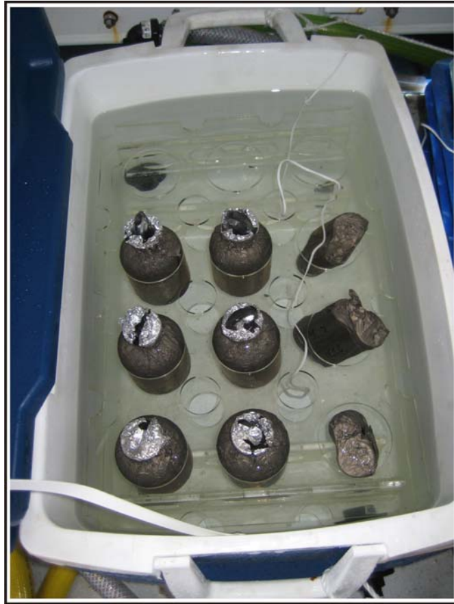
Figure 2.3. Incubator and samples for SOD and vial incubations. Seawater flowed continuously through the incubator maintaining temperatures within 0.1° C of sea surface temperature (SST).
