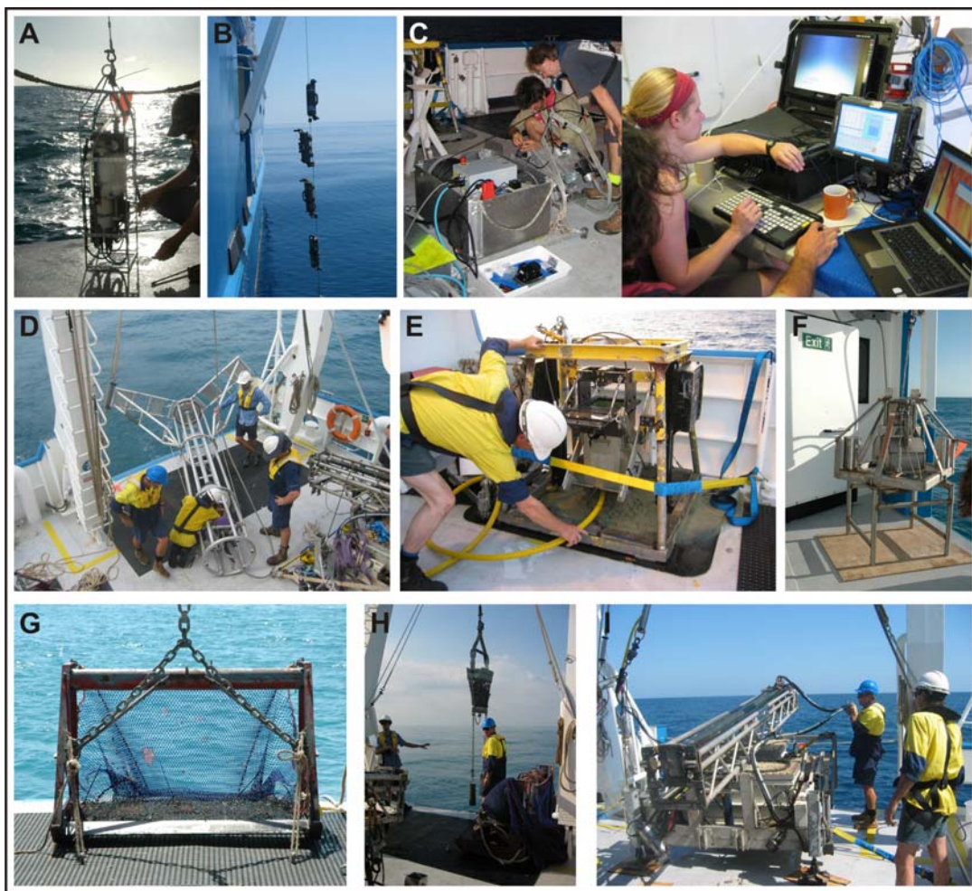
Figure 2.1. Sampling gear used on the survey, including: A) CTD, B) niskin bottles in series, C) video camera and characterisation equipment, D) vibrocorer, E) boxcorer, F) Smith-McIntyre grab (shipek grab not shown), G) benthic sled, H) rock dredge, and I) rotary corer.
