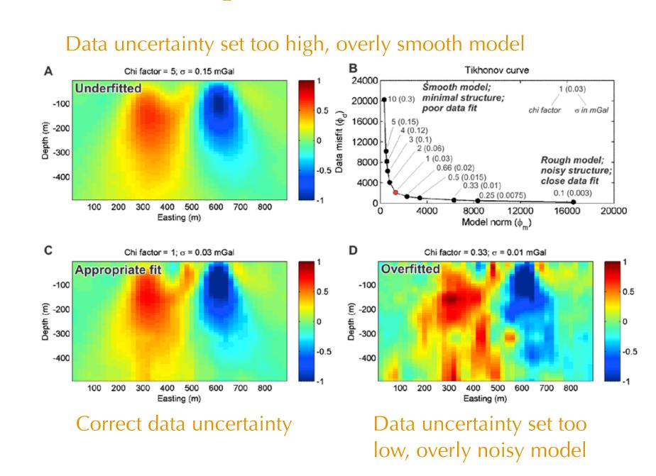
Geophysical data must be assigned an uncertainty, expressed as a standard deviation. This includes uncertainty in measurements and approximations due to using discrete cells and model volume.
