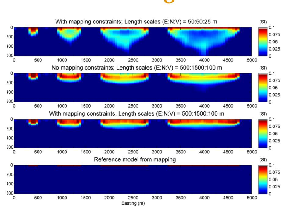
Smoothness provides geological continuity where geophysical data are sparse or provide limited information.
