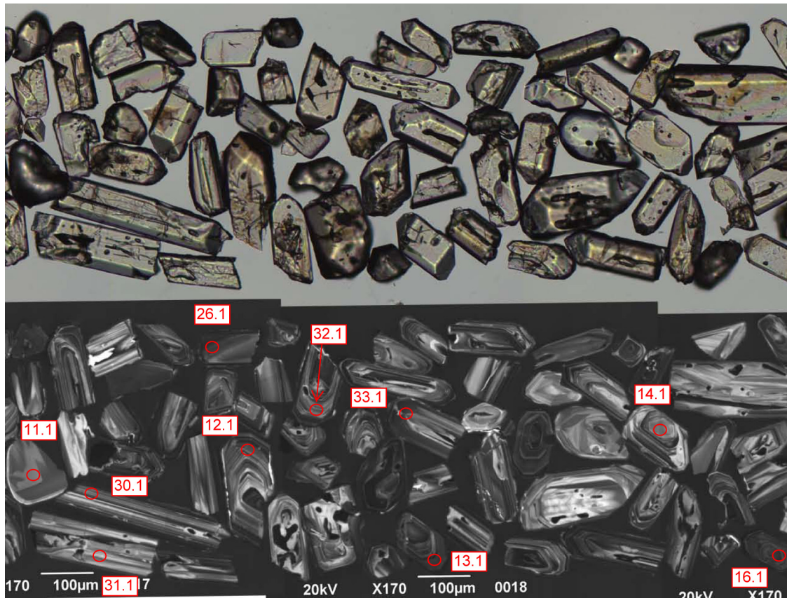
Figure 16: Representative zircons from the 'leucogranite phase' of the Lockhart Igneous Complex (GSNSW 8827JAF0837, GA 1974958). Transmitted-light image is shown in the upper half; cathodoluminescence image in the lower half. SHRIMP analysis sites are indicated, and labelled with grain and spot number.
