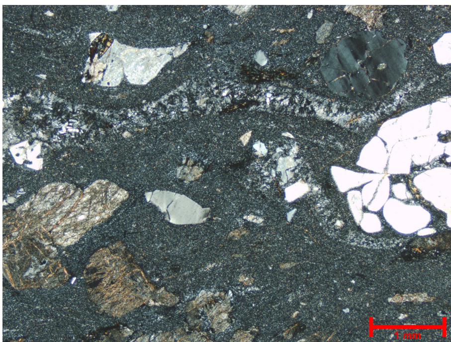
Figure 30: Representative photomicrograph (in cross-polarised light) of the Croppies Gunyah Rhyolite (GSNSW 8827CJS0070, GA 1989476). Densely welded rhyolitic ignimbrite contains crystals of quartz (right), altered plagioclase (lower left), K-feldspar (top right), and rare chloritised biotite (top centre). The finely microcrystalline, welded matrix contains lenses of more coarsely microcrystalline material (upper half), which are interpreted as strongly flattened pumice clasts.
