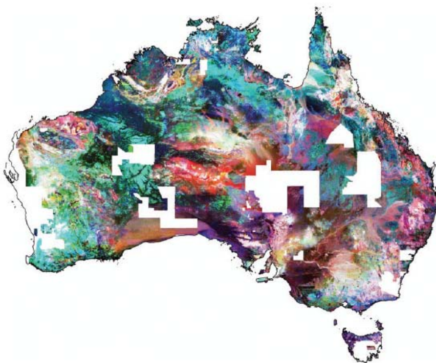
Figure 2. Ternary image (K-red, eU-blue, eTh-green) of Australia derived from the new levelled National Radioelement Database (Minty et al. , 2009b).
