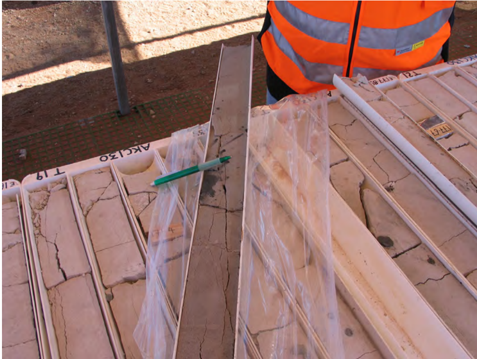
Figure 5. Sandy diamictite zone from Four Mile West (drill hole AKC130, ~183—148 m). Note dark grey patches of framboidal pyrite (2001026).
