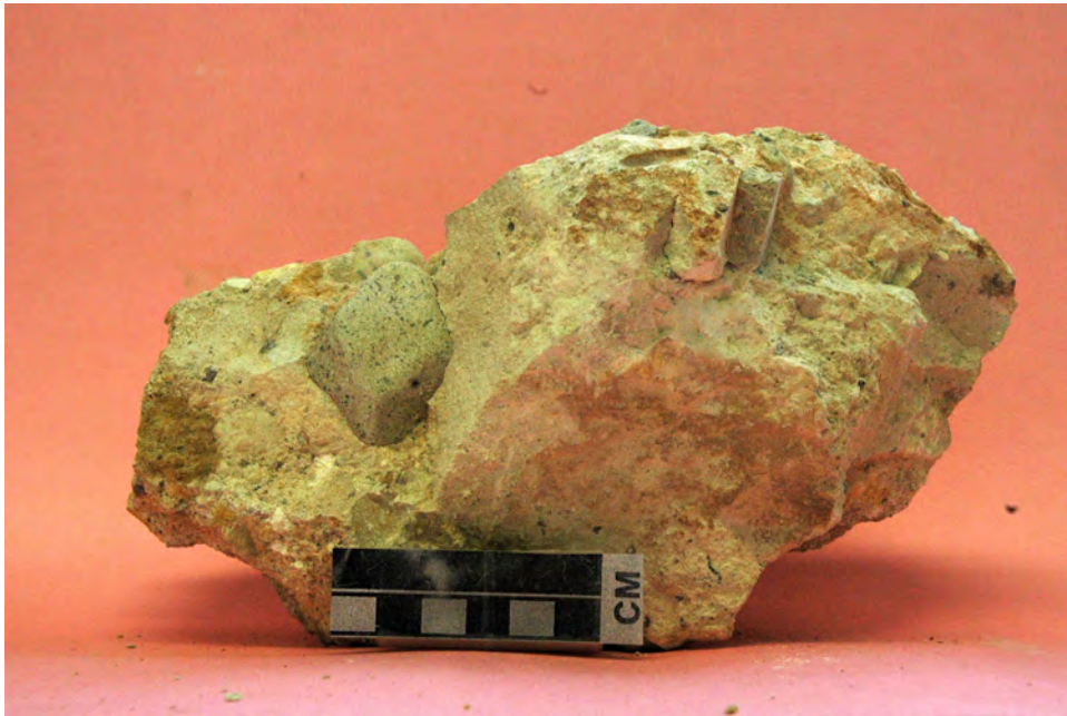
Figure 1. Photo of hand sample of matrix supported Cretaceous diamictite (Dead Tree section 1987605).
