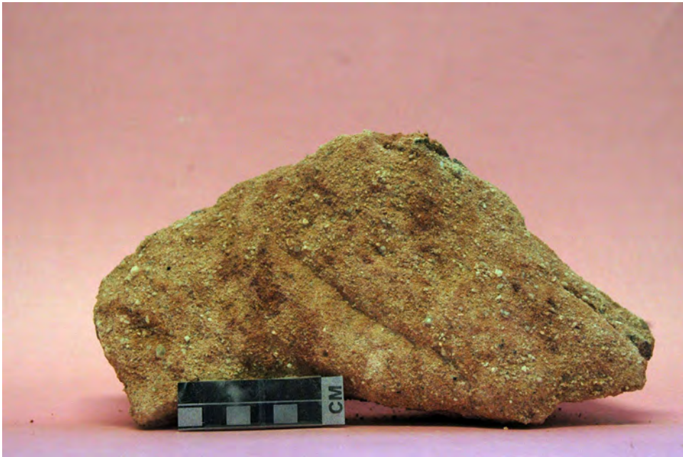
Figure 9. Photo of hand sample of coarse grained sandstone from the Eyre Formation (1987606).
