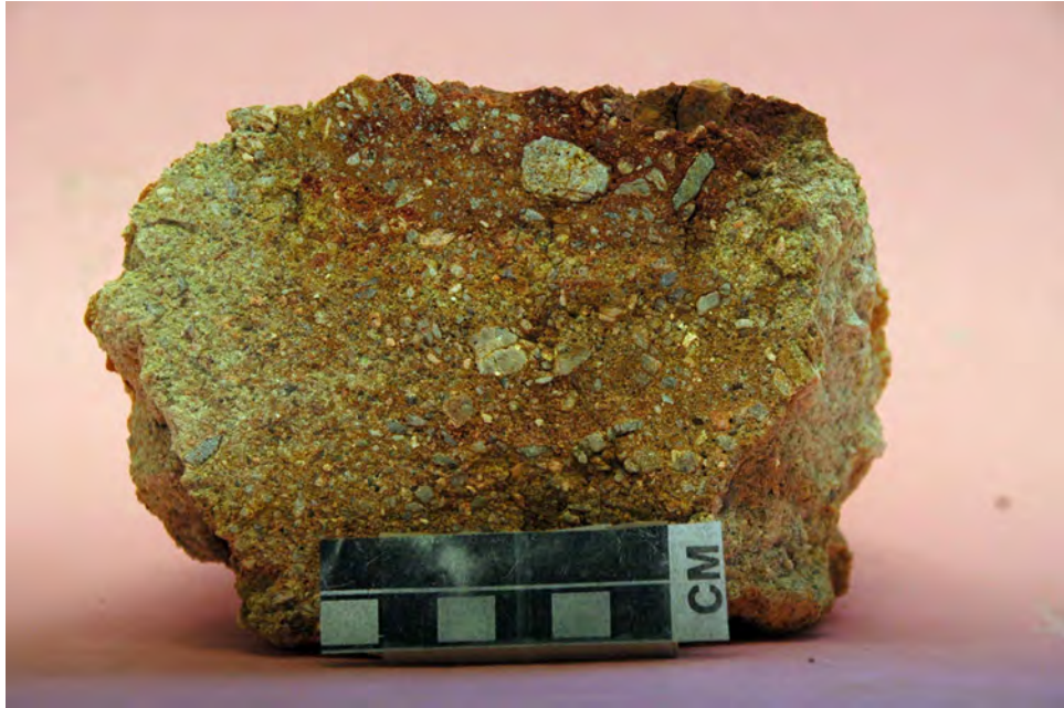
Figure 13. Photo of hand sample of coarse-grained sandstone from the Namba Formation (1987604).
