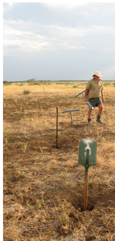
Bottom sample is collected from several auger holes.
