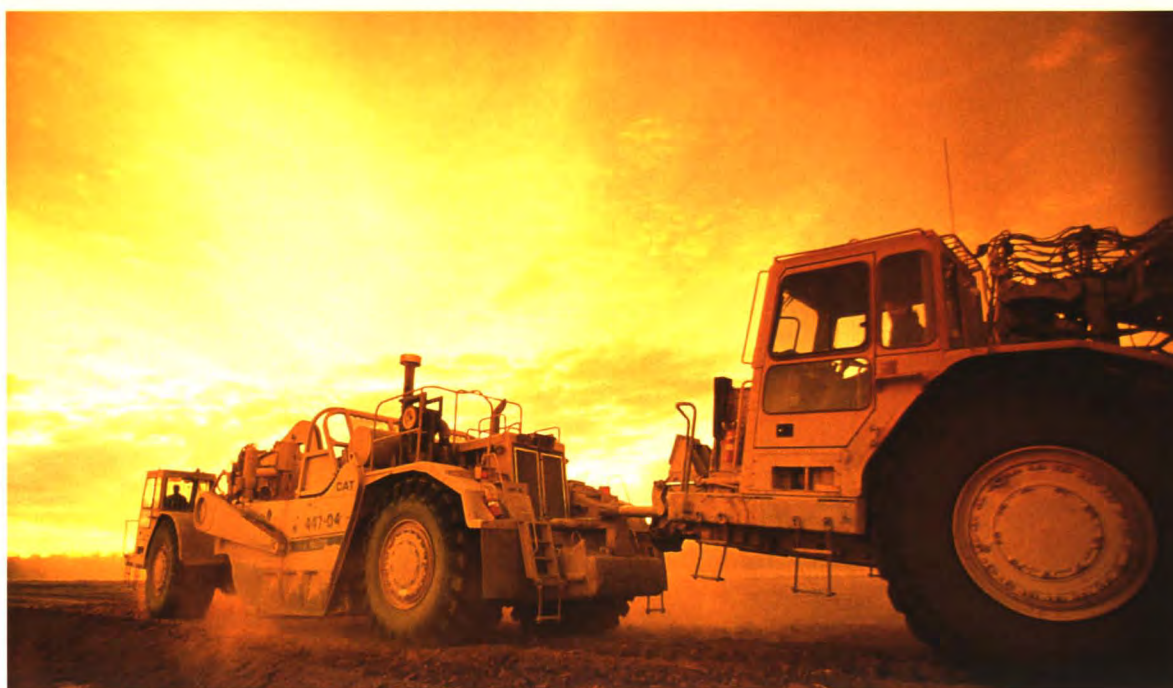
Plate 1 Scrapers removing overburden at the Weipa Mine on Queensland's Cape York Peninsula
