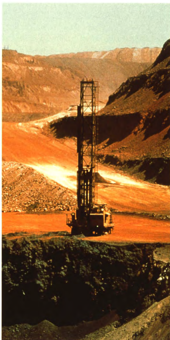
Plate 4 A blast hole drill at BHP Iron Ore's Mount Whaleback iron ore mine, Western Australia
