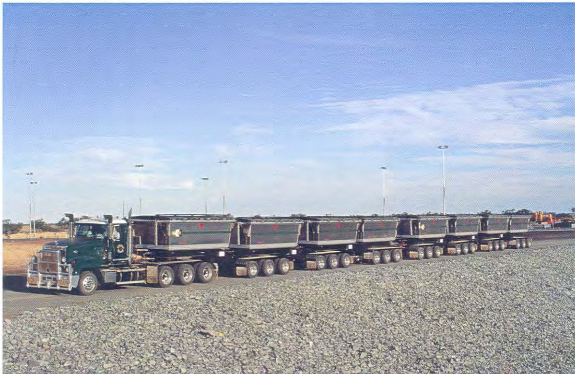
Plate 5 Then Cannington ICON (Innovative Combination of the North) is a 233 combination used to transport Cannington concentrates to the Yurbi rail loading facility
