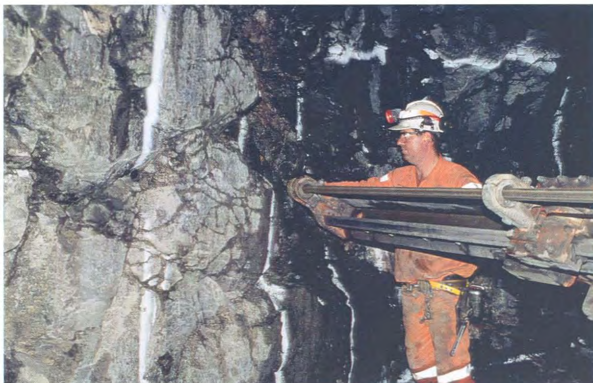
Plate 4 Underground drilling of blast holes at the Cannington project, Queensland Photograph courtesy of BHP Minerals
