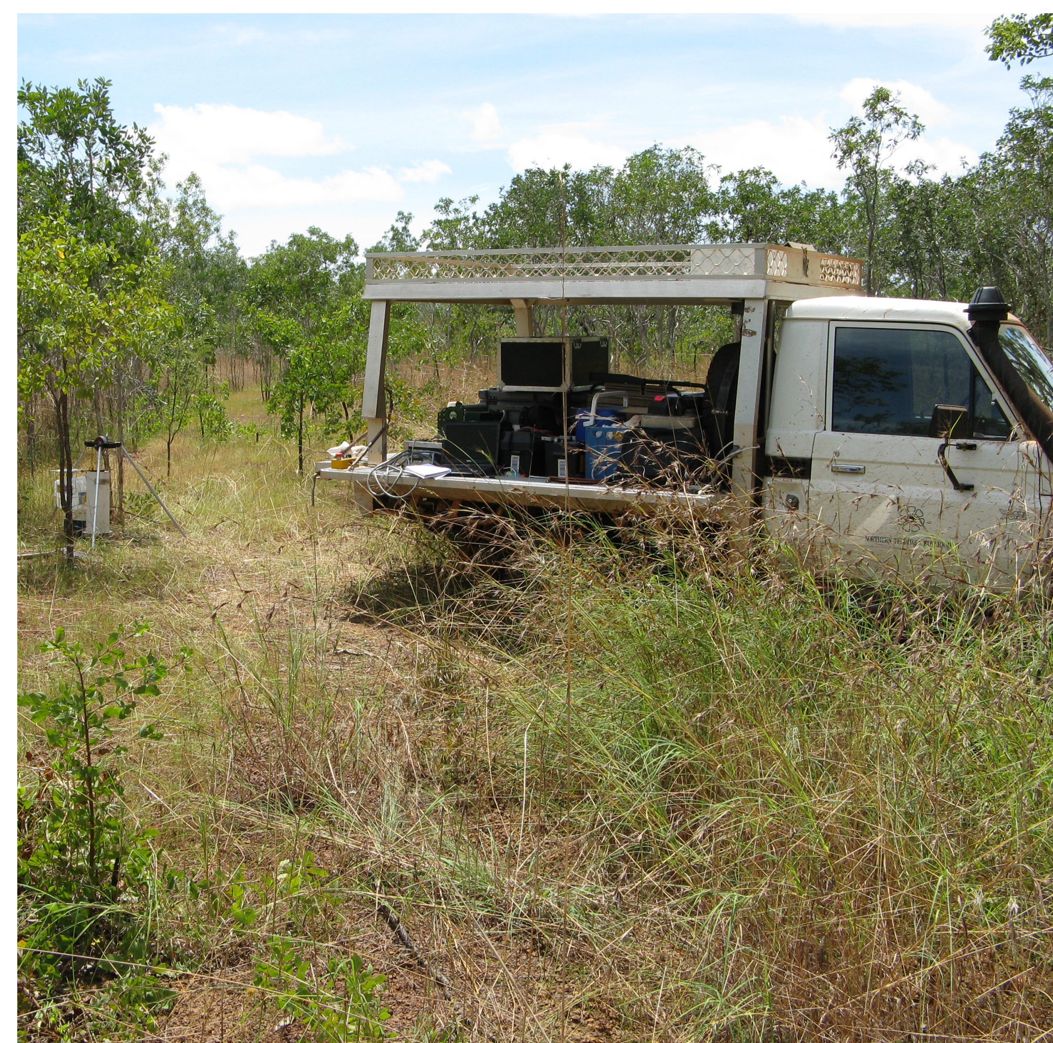
Figure 3. Geoscience Australia undertook induction conductivity logging in the Pine Creek region. Conductivity logs were processed and used as input for forward models, and for interpretations.
