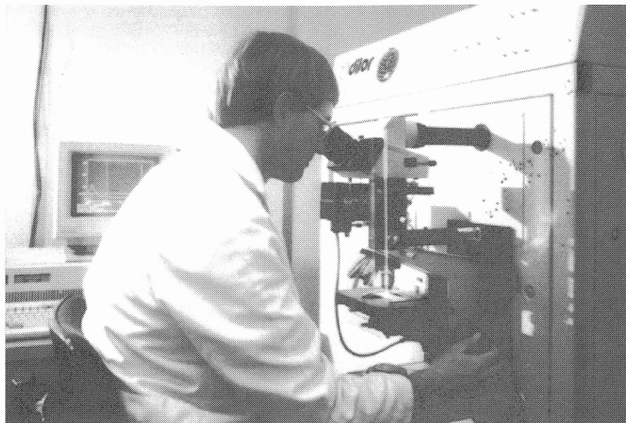
Fig. 16. Dr Terry Mernagh analysing a sample of rock with AGSO's Microdil 28 laser Raman microprobe.
