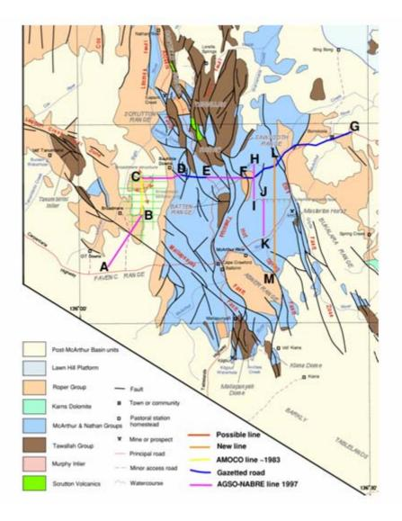
The regional E-W line is designed to acquire deep seismic data to provide a continuous profile of the crust through the Batten Trough. The regional E-W line recorded went from point **C** to some 20 km east of the Emu Fault or some 10 km west of point **G** near Borroloola. The N-S line recorded is line **H** - **I** as shown on Figure 1.
