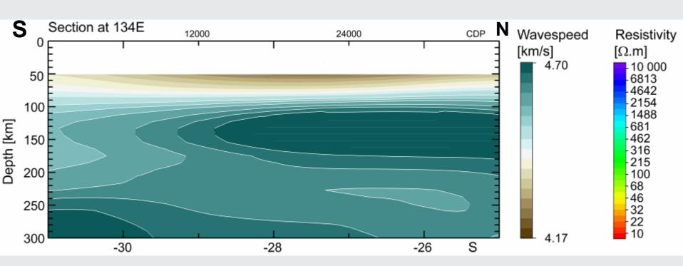
Fast seismic shear-wave speeds to ~200km depth = approximate base of lithosphere
