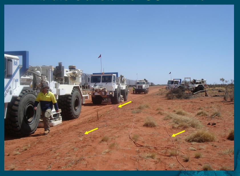
Split spread with maximum 6 km offset 300 channels at 40 m intervals 80 m VP interval
