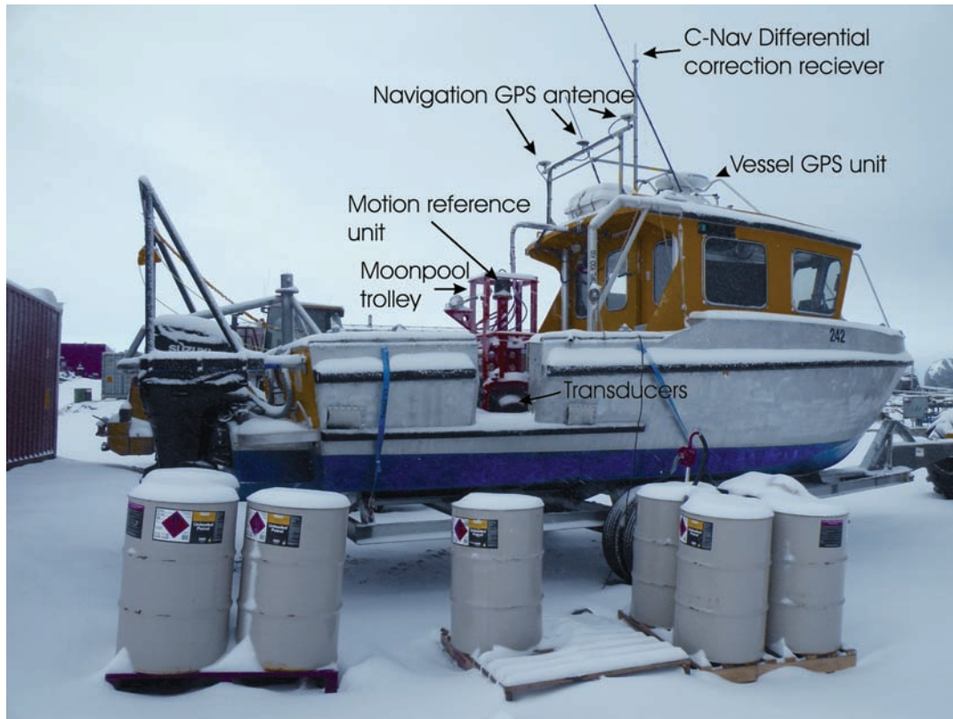
Figure 17: Set up on the RV Howard Burton. Transducer heads were attached mechanically to the motion reference unit and the whole trolley lowered into the moonpool and locked in place. Video winch sat aft of the moonpool trolley with the video deployed on the aft davit
