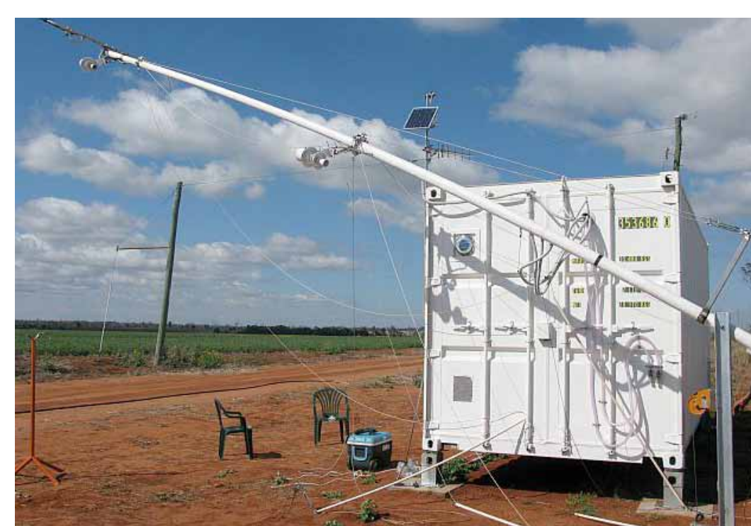
10 m (fibre-glass mast) being winched up/down; aspiration inlets at 5 m and 10 m heights; and meteorological sensors at 10 m.
