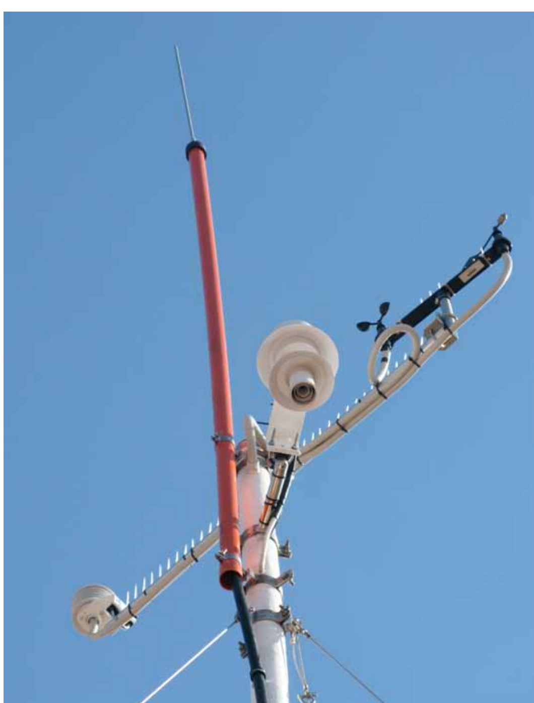
Top of 10m fibre-glass mast showing aspiration inlet; meteorological sensors and lightning rod. (The other inlet is at 5 m).
