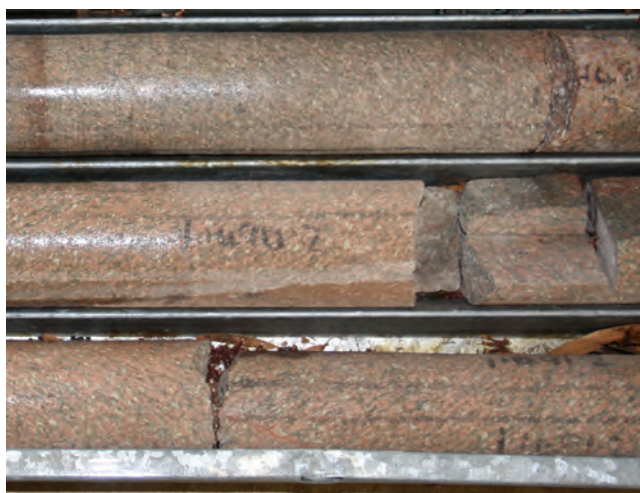
Figure 11.1. Representative core of unnamed granite HU10JAW037 in Phillip 2 drillhole.
