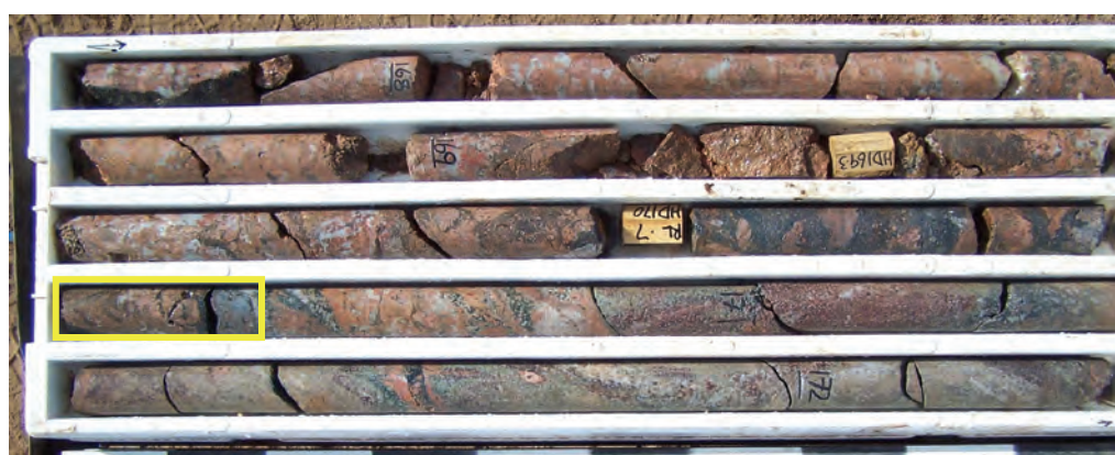
Figure 6.17: Drill core from MN102, Armchair deposit, showing hematitic breccia within granitic breccia, and location of Re-Os sample MN102 170.5 (yellow outlined box). Depths of core in tray extend from 167.7m to 172.3 m. Scale bar beneath core tray in 10 cm intervals. Photo courtesy Marathon Resources.
