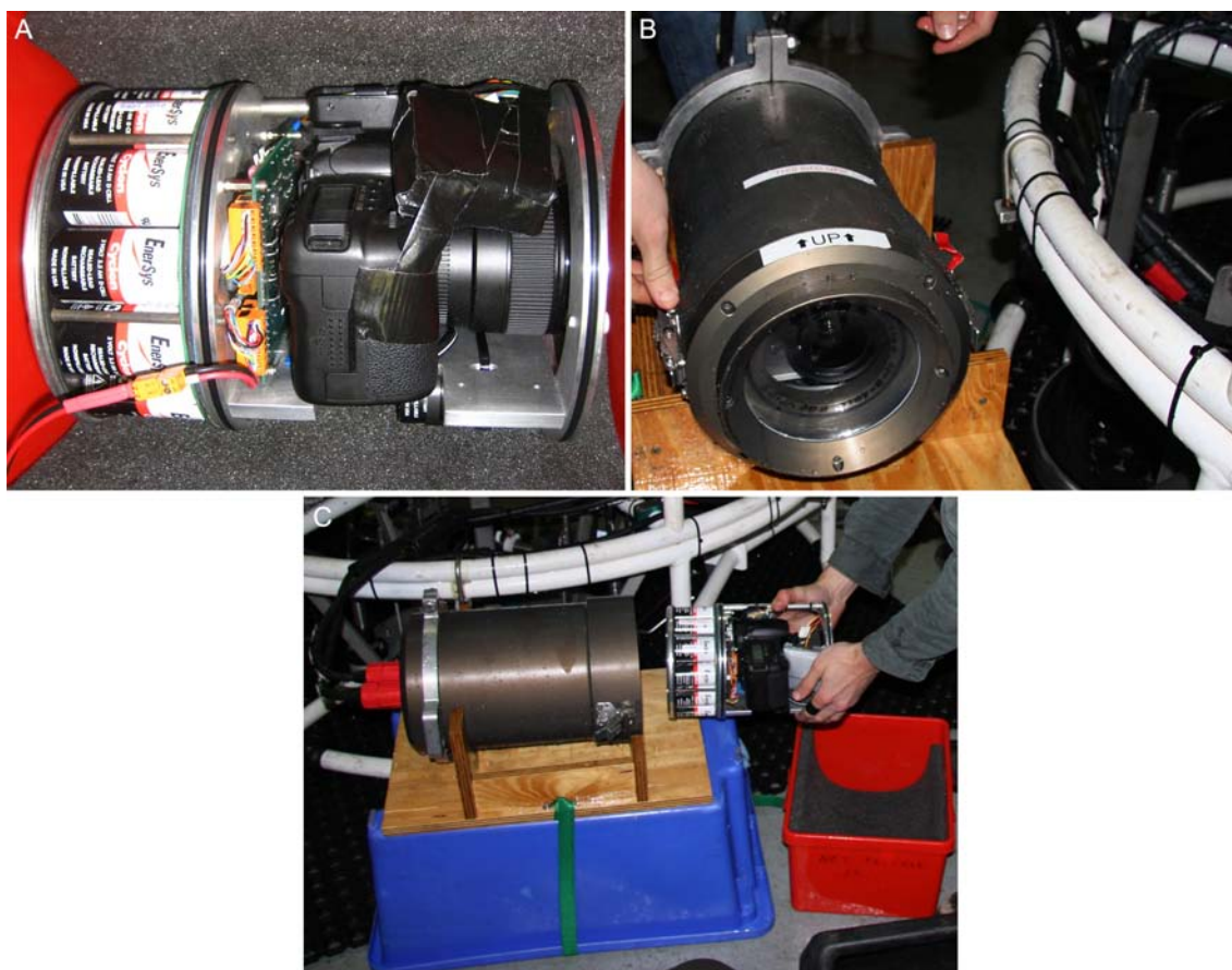
Figure 9: A) Canon EOS 20D SLR 8 megapixel stills camera fitted with a Canon EF 35mm f1.4 L USM lens and powered with a 28V 2.5Ah cyclone SLA battery pack. B) Stills camera within the 2500 m-rated flat port anodised aluminium housing. C) Stills camera being removed from the housing which is connected to the strobes using Brantner Wetconn series underwater connectors (thick black cables with red connectors).
