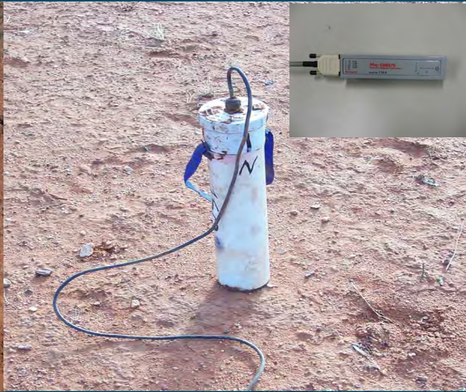
3 component Fluxgate magnetometer
