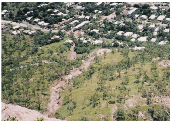
Figure 7: Debris flow which ran into houses near the base of Castle Hill, Townsville.
