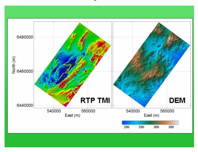
As part of the survey, magnetic data and a high-resolution digital elevation model (DEM) were also acquired. Due to line spacing and terrain clearance factors, the magnetic data do not improve upon the existing 100m line spaced data. The AGG DEM, based on laser ranging measurements taken by a scanner that acquires a swath of data rather than a single profile, is a substantial improvement on the DEM based on radar altimeter measurements from the 100m mag-spec surveys.
