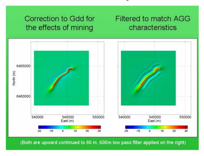
The corrections for mining activity calculated at the flying height amount to a narrow anomaly with peak amplitude of around 30 Eo. Before adding this response to the observed data, the anomaly was filtered to remove short wavelengths, in keeping with the characteristics of the AGG data. The filtering broadens the anomaly and reduces the peak amplitude.
