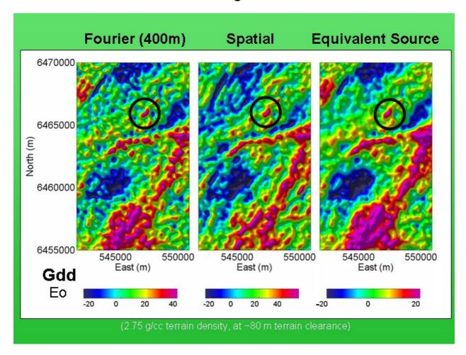
The three different transformations are based on a Fourier domain procedure, a spatial convolution filter and an equivalent source inversion procedure. Robust features have a similar appearance in all three images. Noise related features vary significantly in appearance across the three images.
