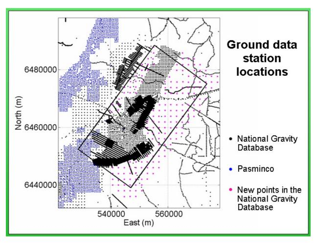
The coverage of ground gravity stations is extremely variable in spacing and quality. To assist in the evaluation of the AGG data, around 200 additional stations were acquired for Geoscience Australia. These data will be available at the end of July.
