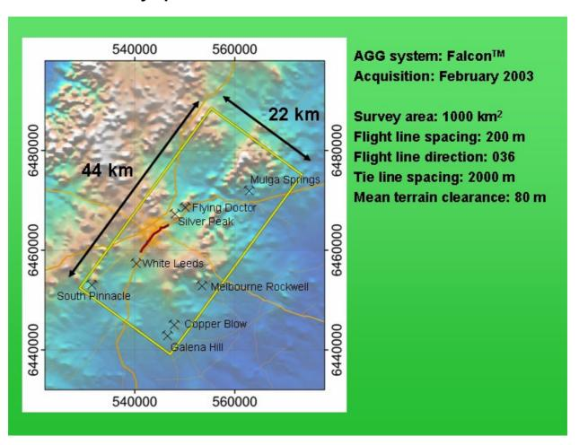
The acquisition phase of a  $Falcon^{TM}$  AGG survey is similar to that of a mag-spec survey. Flight lines were spaced 200m apart, with tie lines spaced at 2000m intervals used for levelling of the data. A limited amount of QC was carried out on site, with the majority of the processing being carried out by BHPBilliton in Melbourne.
