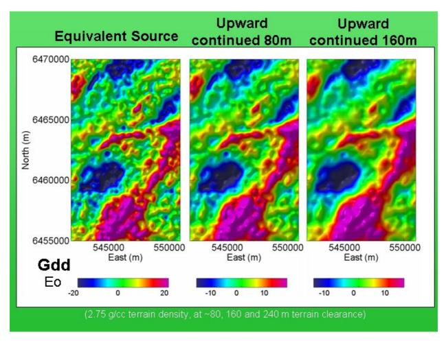
Upward continuation is another form of low pass filtering that can be applied to the data. The optimum trade-off between noise amplitude and spatial resolution is dependent on the application and the preferences of the interpreter.
