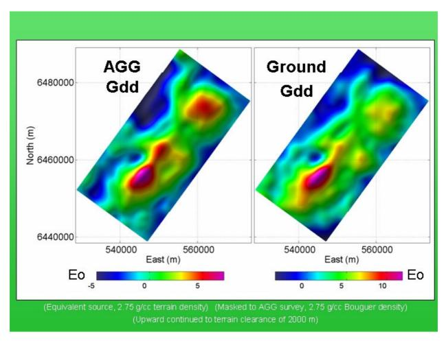
The longer wavelengths in the ground and airborne data can be more easily compared after the short wavelengths have been attenuated by upward continuing both to a height of 2 km above the surface. An analysis of the long wavelengths may seem academic when most of the focus is on short wavelength discrete targets. However, these wavelengths are important when the data are used for mapping, and at some point in the future, when surveys are joined into regional compilations.
