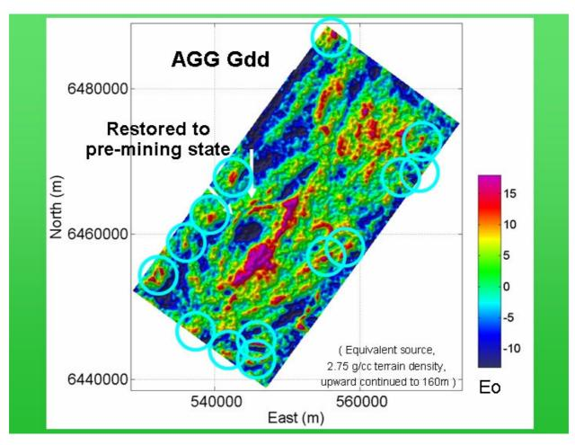
The accuracy and sample spacing of the airborne data is sufficient to identify a number of features with geometry and amplitude characteristics that are similar to a prediction of the premining response of the Broken Hill orebody.
