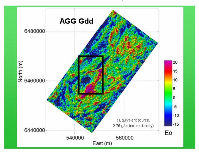
The transformation from measured horizontal gradients to vertical gravity or vertical gravity gradient can be done using a number of mathematical procedures that are described by BHPBilliton as being "different in their underlying assumptions and treatment of noise". Three versions of the vertical gravity gradient are provided. These will be illustrated using a subset of the survey data.
