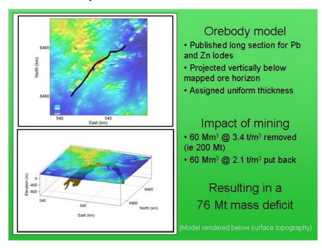
What is the gravity signature of a significant base metal deposit? Ordinarily, you would turn to observations over a known deposit such as Broken Hill for the answer. But in this case, the gravity response has been substantially modified by mining activities. An estimate of the changes has been made and added to the survey data to produce an image of the pre-mining gravity response.
