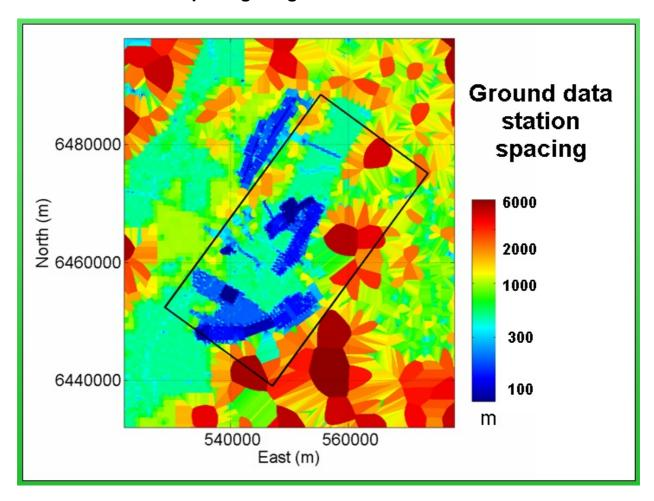
Prior to the acquisition of the new ground stations, there were regions within the survey area where the station spacing was around 6 km as indicated by the deep red colour.
