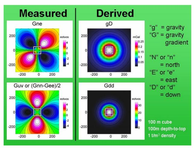
For engineering reasons, the Falcon AGG system actually measures the horizontal gradient quantities Gne and Guv. The plan view response for these quantities for a 100m cube buried at a depth of 100m is shown on the left<sup>1</sup>. These measured gravity gradients have quadrapole response functions that are quite complex even for simple source geometries such as the example shown here.
