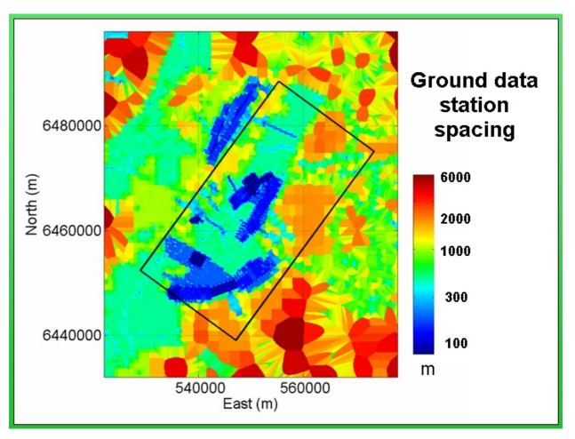
The new gravity data closed down the maximum sample spacing from around 6 km to 2 km and were important for evaluating the long wavelength characteristics of the AGG data.
