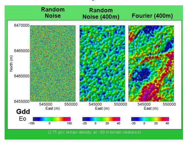
Although the raw data are not available for inspection, it is thought to be contaminated by noise spikes induced by turbulence. This was simulated on the left with a grid of random Gaussian noise that was then low pass filtering in the same manner as has been applied to the Gdd data derived via the Fourier procedure. This resulted in a texture that is very similar to the texture observed in the survey data.
