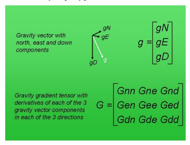
Gravity is a vector quantity that can be described by 3 components: one in each of the north, east and down directions.
