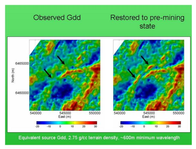
Vertical gravity gradient data from a portion of the survey is shown on the left. The corrections for mining activities have been added on the right. There are distinct highs over the northern and southern parts of the orebody which hosted the bulk of the reserves.
