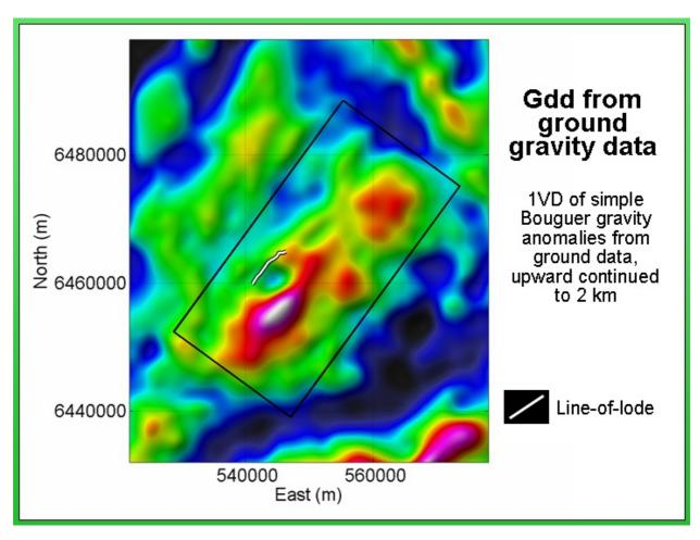
The AGG survey surrounds the prominent Thorndale and Mt Vulcan gravity highs immediately to the east of Broken Hill. The elongate gravity low to the south underlies part of the Redan sequence. The NW trending low to the north of the survey is associated with a tongue of Adelaidean sediments and with upper parts of the Willyama Supergroup. The elevated plateau to the west of the survey is associated with the central portion of the Broken Hill Block.
