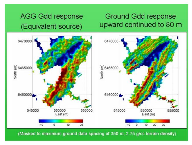
To evaluate the short wavelength resolution of the airborne data, an image of the vertical gravity gradient derived from ground data covering a small portion of the airborne survey is shown on the right, upward continued to 80 metres.
