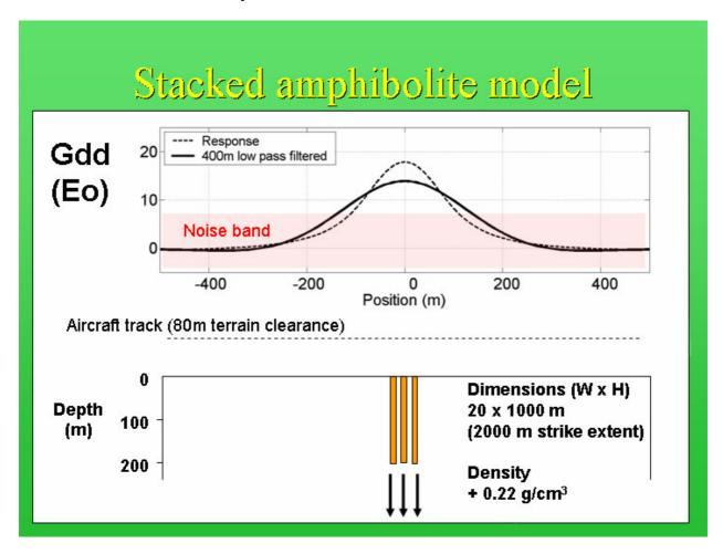
There are numerous relatively dense amphibolite horizons in the survey area. A stacked sequence with a combined width of around 60 m would produce a similar anomaly to the ore body.
