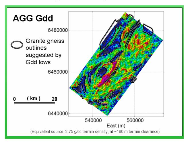
The outlines of granite gneiss on this slide have been modified in accordance with the extent of gravity gradient lows.
