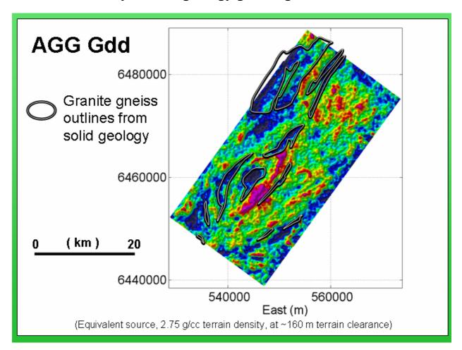
These boundaries have been transferred as an overlay onto a vertical gravity gradient image. As expected from the analysis of density measurements, there is a reasonable correspondence of vertical gravity gradient lows with granite gneiss bodies. However there are also significant discrepancies.
