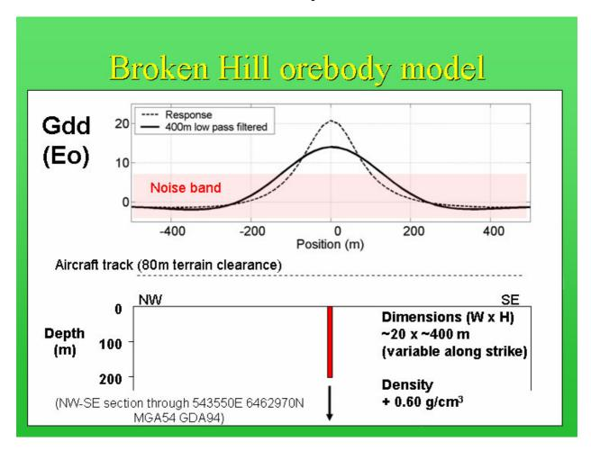
As well as calculating the changes brought about by mining activities, the vertical gravity gradient response of the original ore body was calculated. A profile from north of the Zinc Corp. shaft is shown.
