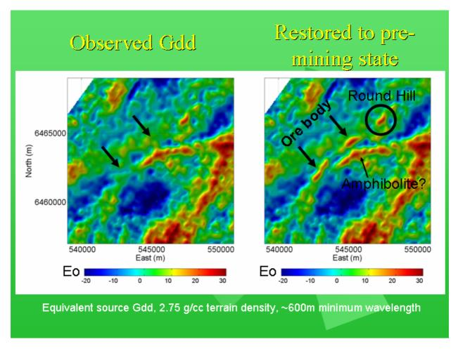
Vertical gravity gradient data from a portion of the survey is shown on the left. The corrections for mining activities have been calculated and added to the image on the right. There are distinct highs indicated by the arrows over the northern and southern parts of the ore body which hosted the bulk of the reserves.
