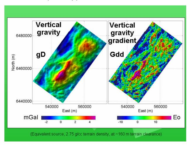
The principal survey products are grids of vertical gravity, gD, and vertical gravity gradient, Gdd. The latter is simply the first vertical derivative of vertical gravity.
