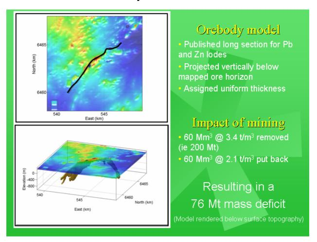
The observed gravity response in the vicinity of the Broken Hill ore body has been substantially modified by changes in mass distribution brought about by mining activities. As a result, there are two nagging questions that surround this gravity survey;
