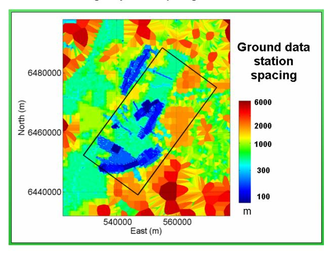
The ground gravity data within the survey area have variable station spacing, from less than 100 m to around 2 km. Except in the areas shown in blue, this coverage lacks the detail to detect features of direct interest for base metal exploration. The AGG survey has revolutionised the level of detail, reducing the effective sample spacing down to a uniform 2 or 3 hundred metres.
