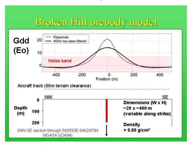
We have seen that the original Broken Hill ore deposit would have produced an anomaly above the noise level. But what other geological features would give rise to similar vertical gravity gradient anomalies?
