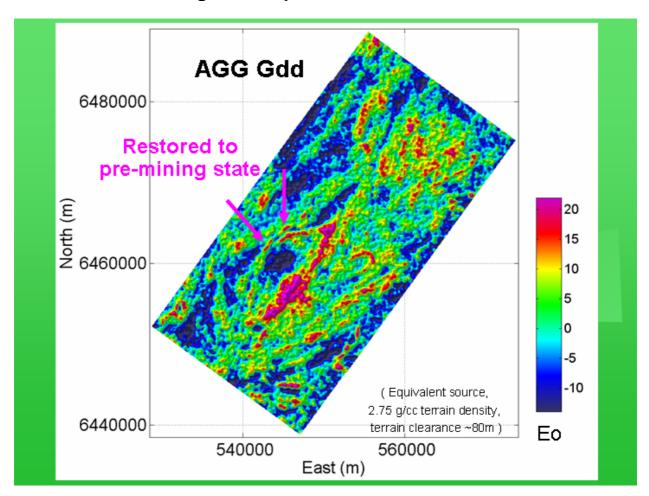
Restoration of the gravity response for the impact of mining indicated that had the survey been flown prior to mining, the Broken Hill ore body would have been detected as a target for follow-up.
