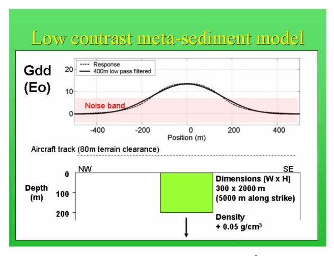
A 300 m wide meta-sediment unit with density elevated by just 0.05 g/cm³ would also give rise to a similar anomaly. Without careful sampling and measurement of density, it would be difficult with this scenario to reconcile drilling results with the source of the anomaly, and an explorer might be left wondering where the dense target disappeared to.
