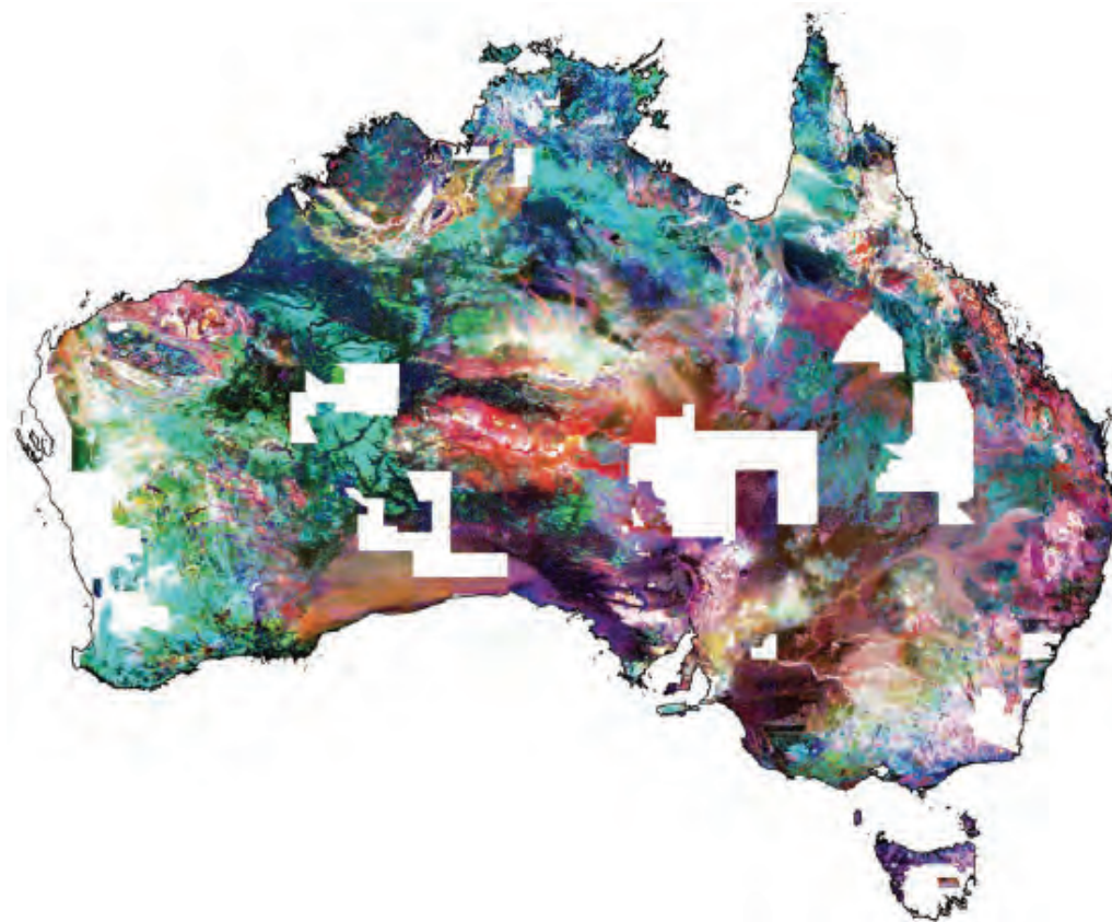
Figure 2. Ternary radiometric image (K-red, eU-blue, eTh-green) of Australia derived from the new levelled National Radioelement Database (Minty et al. , 2009b)
