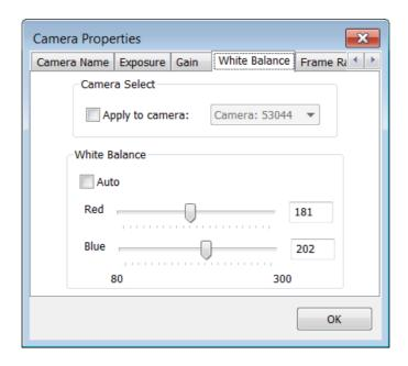
White balance can be used to remove unrealistic colour casts from the images. The default values of Red = 181 and Blue = 202 was found to be the most suitable.
