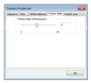
Field trials suggested that four consecutive frames are necessary to capture an entire house with an average frontage of 20 metres using 12.5 mm lenses. With two cameras attached to the laptop, the maximum frame rate is four frames per second for a GigE 5 megapixel camera. This suggests a maximum vehicle speed of 72 km/h. However, to reduce the
