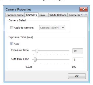
It has been found that setting the exposure time to *Auto* and setting an *Auto Max Time* of 5 ms gives the best exposure results. A maximum exposure time is useful to avoid a long exposure time which can result in blurry images.
