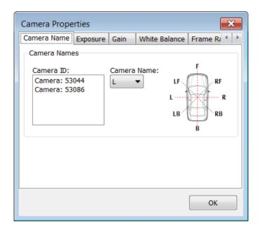
To change a camera name, click on a camera ID and then select a camera name from the drop-down menu. Images are saved in directories named after the camera names and therefore each camera should be assigned a unique camera name, i.e. two cameras cannot have the same name.
