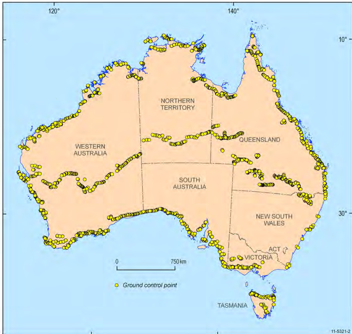
Figure 11: The location of surveyed GCPs for the Australian Geographic Reference Image. 2885 features were surveyed at 737 sites
