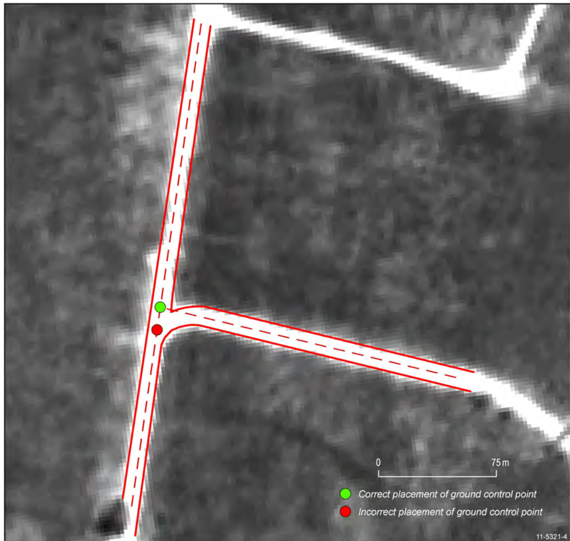
Figure 10: Correct placement of a GCP at an intersection. Solid red lines mark the edge of the linear features and dashed red lines mark the centrelines. The green dot marks the correct placement of the GCP.
