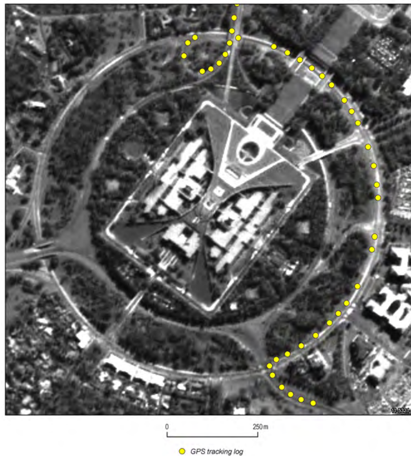
Figure 3: Example of dGPS tracking data overlain on the orthorectified PRISM imagery
