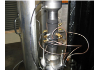
4 multi stage triaxial tests on Paaratte Fm specimens were used to calibrate CRC-2 sonic logs for static mechanical properties. The Paaratte Fm and overburden were broken down into discrete zones of variable Young's modulus, Poisson's ratio and UCS.
