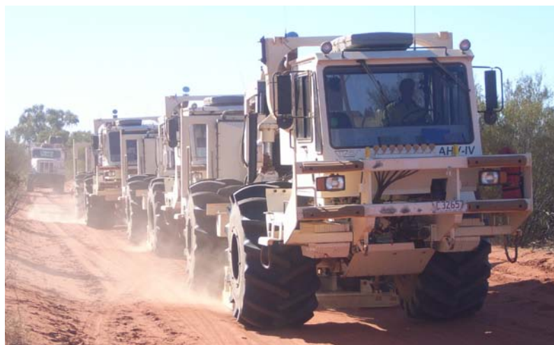
Figure 2. Vibroseis trucks used to acquire onshore seismic reflection data for the Georgina Survey in the Northern Territory.
