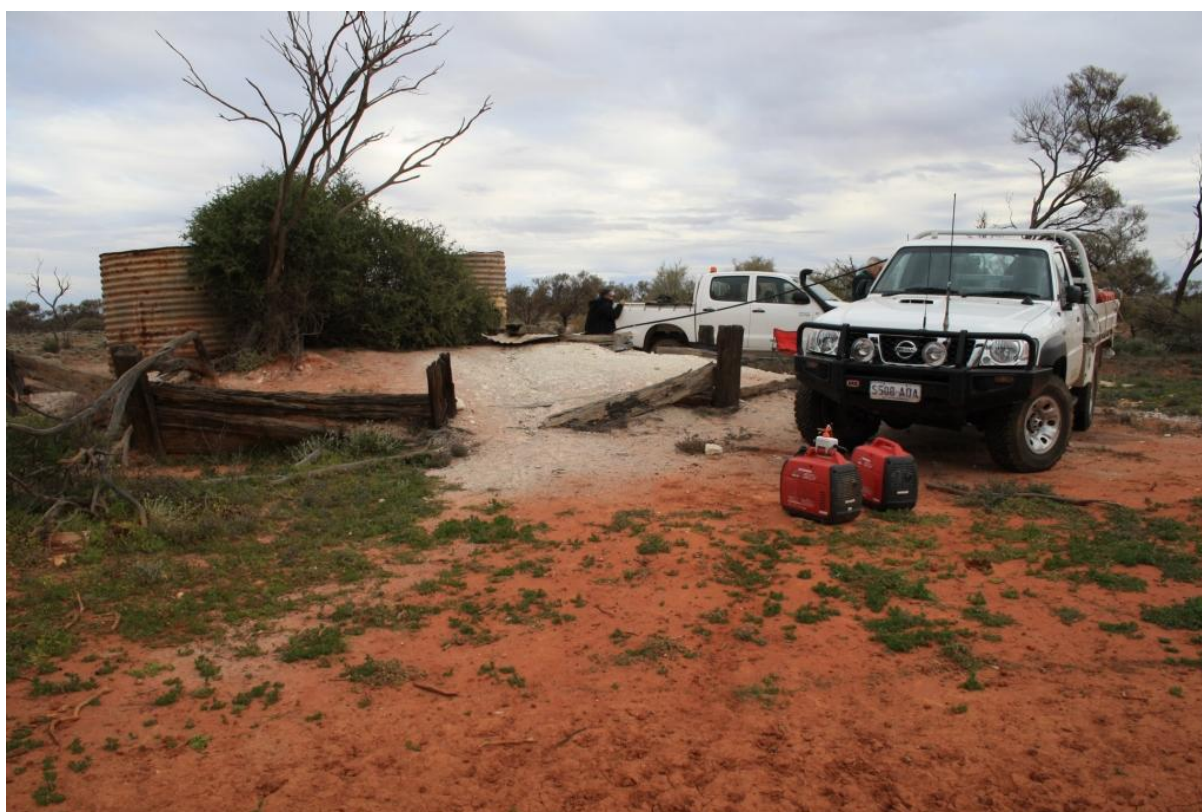
Figure 42: Portable generator system set-up for running the MP-1 pump during groundwater sampling operations in the Kingoonya Palaeovalley during July 2010 (photo courtesy of Tania Wilson, GSSA, July 2010).
