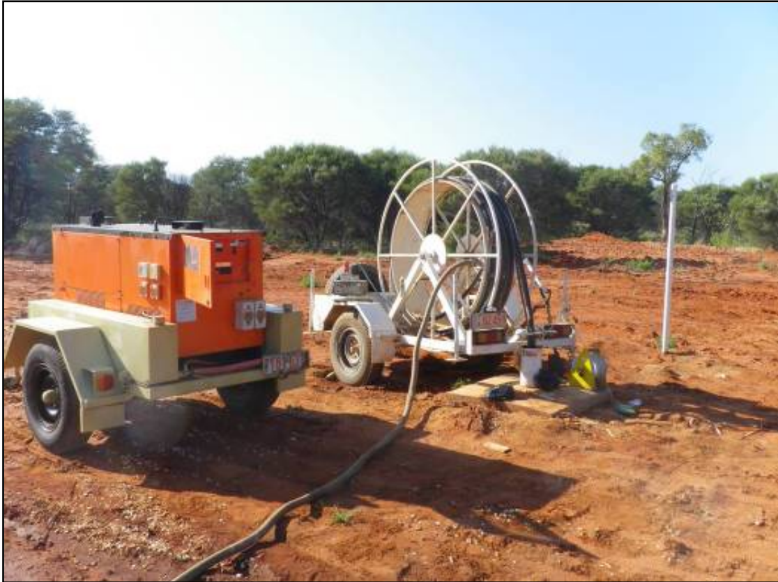
Figure 4.15: Submersible pump reel and generator at bore RN 18594 in September 2010 to collect water samples for ionic and isotopic analysis.
