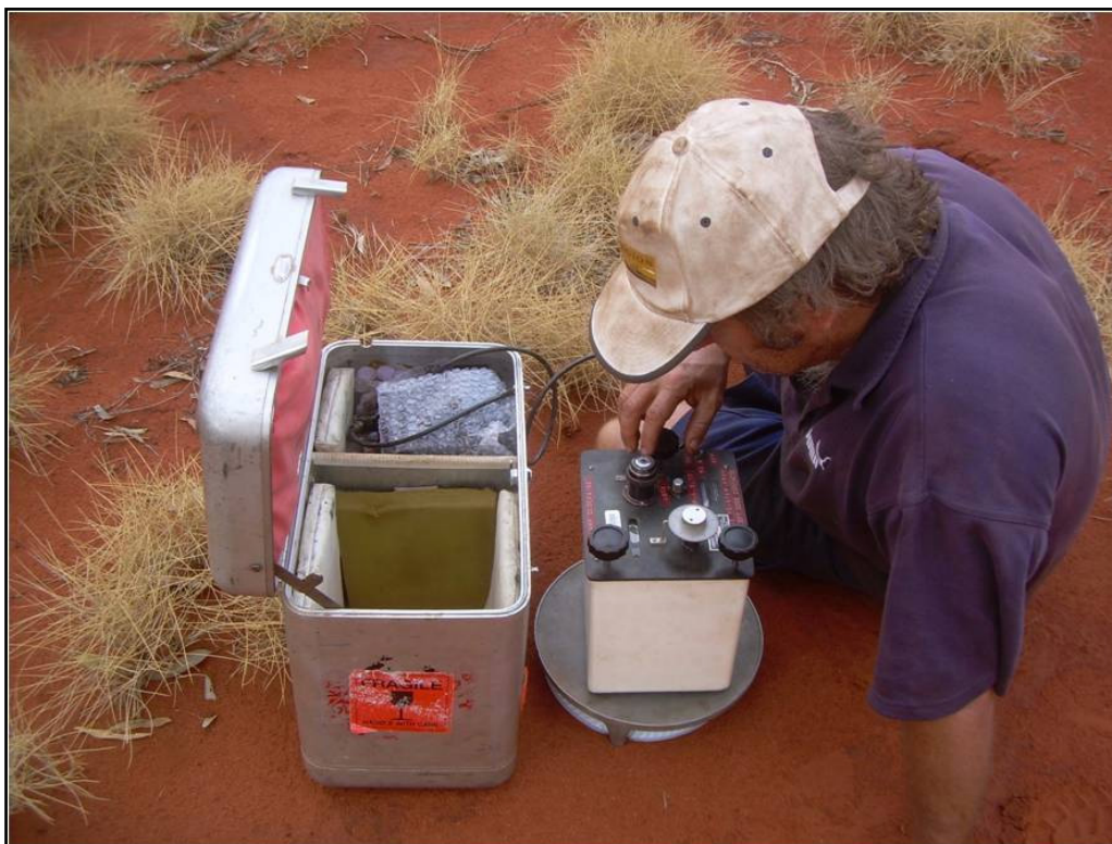
Figure 4.2: Dr John Wischusen of Geoscience Australia collects a gravity reading along the west to east survey line in the Ti-Tree Basin.
