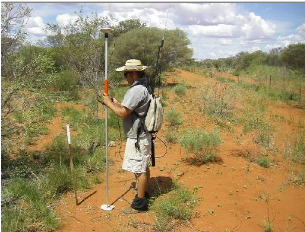
Figure 4.3: Levelling gravity survey stations using DGPS to correct for the influence of elevation on the field-based (raw) gravity readings.
