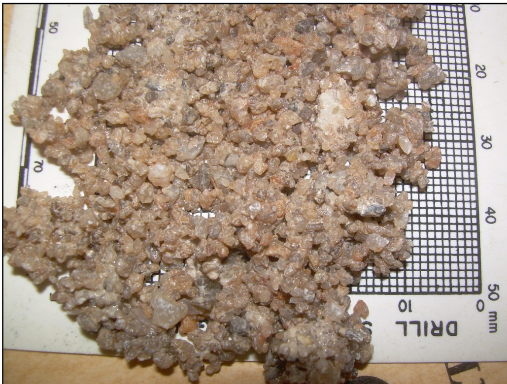
Figure 4.7: Coarse-grained and poorly consolidated sands recovered from RAB drilling of borehole RN 18356 (208–214 metres below surface).
