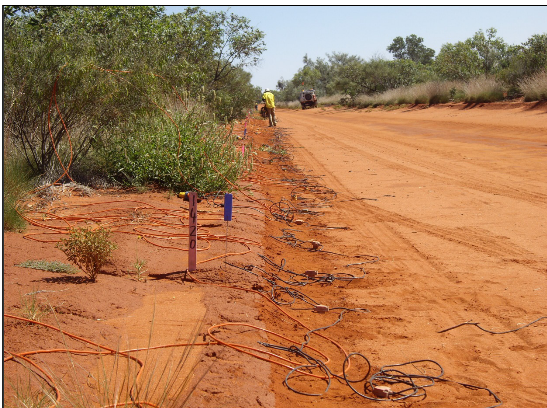
Figure 5.13: Groups of six geophones with 1.3 metre spacing placed along the seismic line.
